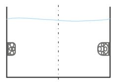
Fig. 23-1 Sensor mounting on the wall
