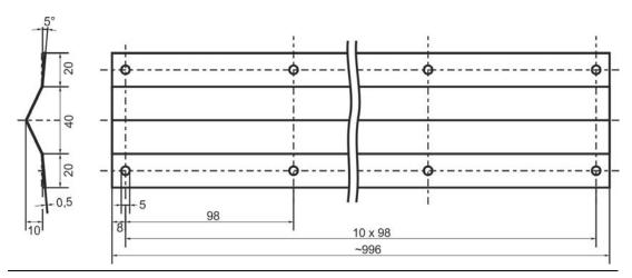
Fig. 23-19 Dimensional drawing cable protection sheet Type ZMS 140
