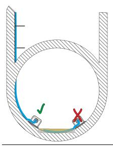
Fig. 23-10 Cable routing for wedge sensor
