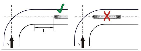
Fig. 22-3 Sensor position behind curves or bends
