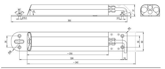
Fig. 15-4 Sensor dimensions PKM-V1xxKL... (with cable cover)
