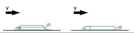
Fig. 22-1 Sensor position in the direction of flow
