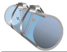
Fig. 42-2 1-Path measurement, path arrangement: "Diametral V"
