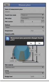
Fig. 34-3 Accept changed measurement place parameters
