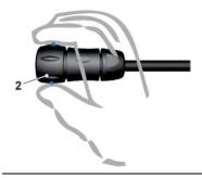
Fig. 25-2 Turning the front ring of the plugs (10-pole/18-pole)
