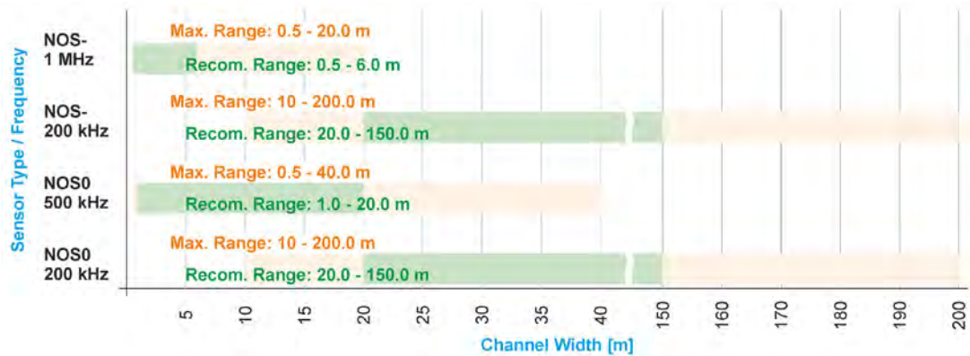
Fig. 18-1 NOS-/NOS0 (rod, (hemisphere) ball sensor) and suitable channel widths
