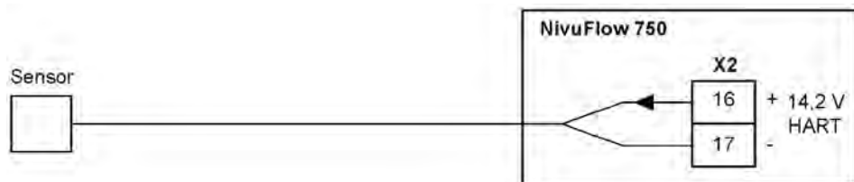
Fig. 23-15 Connection 2-wire sensor for level measurement
