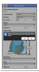
Fig. 33-3 Accept modified measurement place parameters
