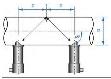
Fig. 24-6 Sensor distance - diameter (principle)
