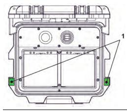
Fig. 15-1 Attachment position for PU stickers
