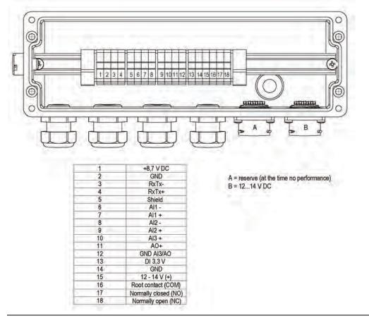
Fig. 27-2 Connector Box terminal wiring
