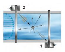
Fig. 20-1 Signal damping due to interfering particles
