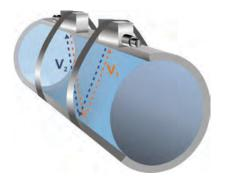
Fig. 38-2 1-Path measurement, path arrangement: "Diametrical V"
