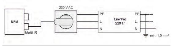
Fig. 25-3 General overvoltage protection for AC power supply
