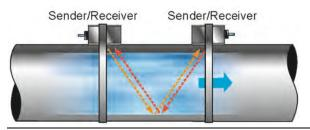
Fig. 24-3 Example "Diametrical V" mode
