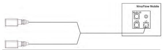
Fig. 25-1 Connection of flow velocity sensors, 1 pair/path
