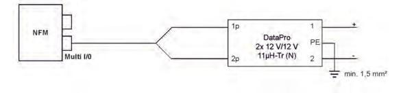
Fig. 25-4 General overvoltage protection for DC power supply
