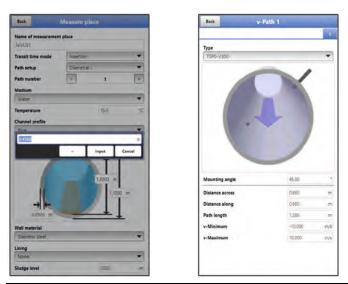
Fig. 24-5 Entering pipe dimensions and mounting angle
