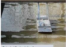
Patented float solution for detection of flow and sedimentation
