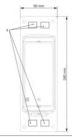
Fig. 23-2 Fastening on a mast using clamps
