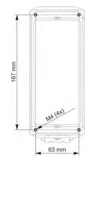
Fig. 23-1 Fastening drilling patterns
