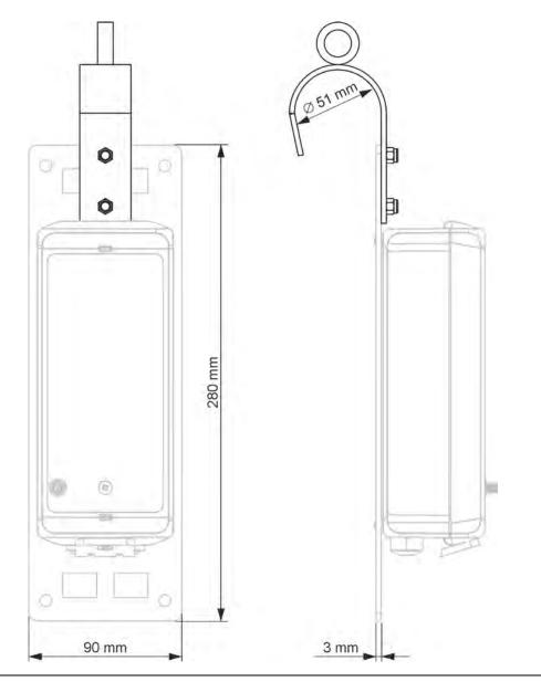
Fig. 23-3 Fastening with bracket on step iron
