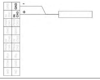
Fig. 28-4 Connecting an active or passive signal transmitter
