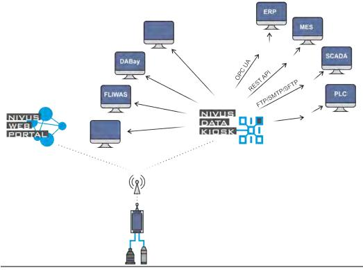
Fig. 20-1 Functional principle of the NivuLink Micro II
