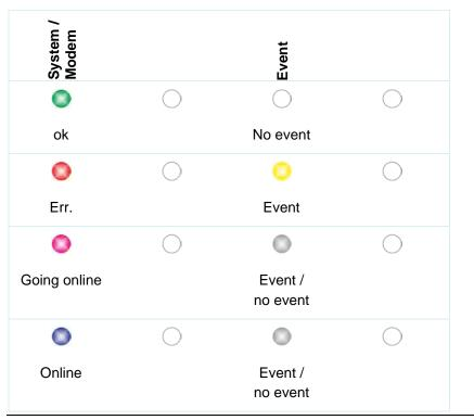
Tab. 6Lighting system of the status LED in shutdown mode
