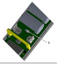
Fig. 24-1 SIM card slot
