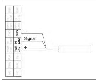
Fig. 28-3 Connecting a 3-wire sensor
