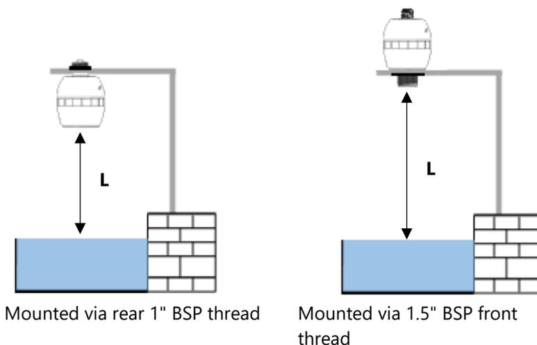
**Closed Vessel Installation**
