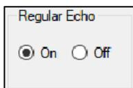
When "Regular Echo" is turned on, the echo status field will highlight red indicating a trace is being obtained and displayed. When obtaining a trace for the first time it will take approx. 7 seconds to retrieve the information. After this the trace will continue to display live information from the sensor every 2 seconds.
