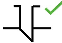
Correct standpipe installation.
