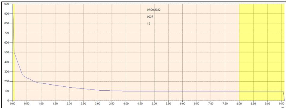
By default, the DATEM in NIVUS Ri-Series sensors is ACTIVE which means it will grow to cover (mask out) any fixed obstructions in front of the current measurement echo.
