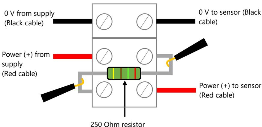
To enable the sensor to work correctly, the power (red) cables from the supply and to the sensor must be wired in series with the 250 Ohm resistor (as seen in the above picture).
