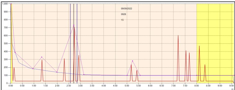
The points can be clicked on and dragged in order to manipulate the DATEM line to cover any unwanted echoes you want to hide from the echo selection algorithm. Once the line is in its final position, click the "Update" button in the DATEM area and the new values will be transferred to the real time DATEM line, and the echo will change like the example below:
