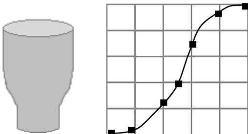
You should enter two level/volume breakpoints at the minimum and maximum levels and several for each place where the vessel has got an arc. You can enter any number of pairs between 2 and 16.
