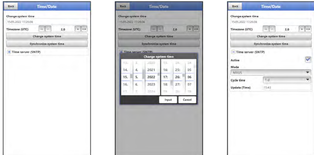
Fig. 41-4 Change system time: automatically and manually
