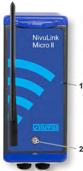
Fig. 32-1 Waking up the NivuLink Micro II / NivuLink Micro II Ex (here: Enclosure S - Special Design)
