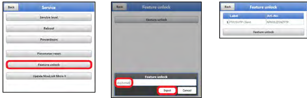
Fig. 41-9 Activation of the licence in the NLG02 display tool
