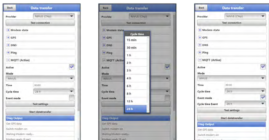
Fig. 42-5 MQTT active / cycle time / event operation
