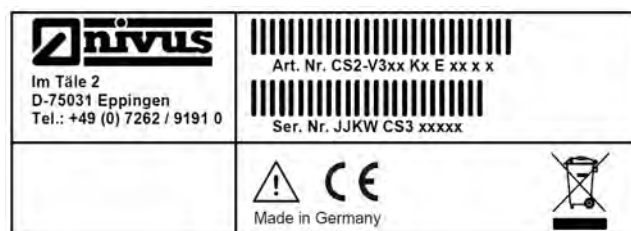
Fig. 4-48 Nameplate for Sensor CS2
