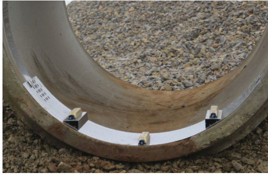
Clamping plates mounted with CS2 sensors
