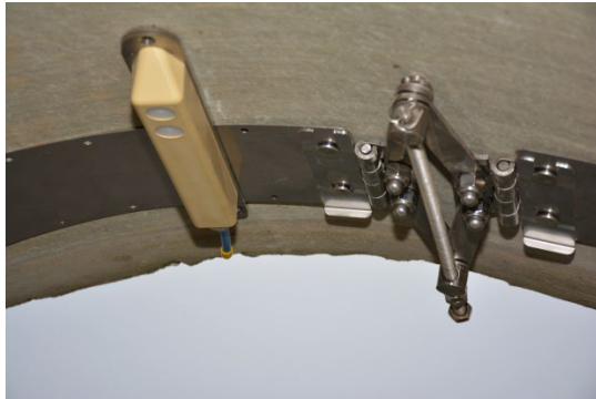
Fig. 14-11 Fully assembled mounting sheets with sensors
