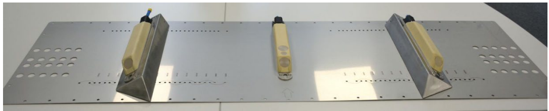
Fig. 14-5 RMS5 mounted horizontally (before installation)
