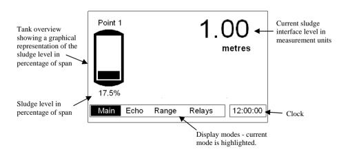
Error messages, such as "Wiper Fault", "Status = LOE" or "Status = Failed" will be displayed on this screen, relating to the point of measure currently being viewed, when a fault condition occurs.
