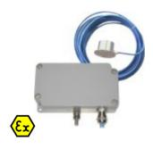
The NDW Inclinometer utilises a capacitive measurement method to measure the inclination (angle measurement) on movable weir flaps. This allows for discharge volume measurement with the aid of the "HydraulicCalculator Plus" transmitter.
