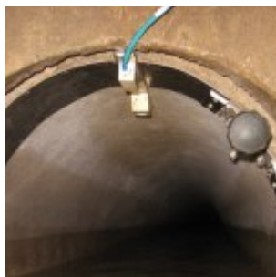
Air-ultrasonic sensor – for detection of low levels e.g. detection of extraneous water
