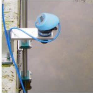
The NivuCompact can be connected to the PCM directly
