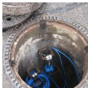
Data logger, mounted in manhole
