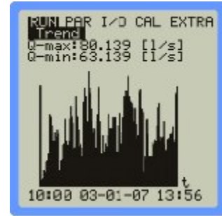
Internal logging options for assessment of the measurement progress on site without additional aids
