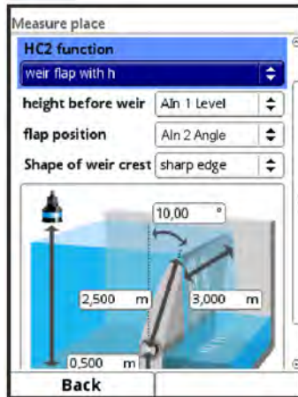
Fig. 34-3 Example of a calculation on a weir flap with impoundage target correction
