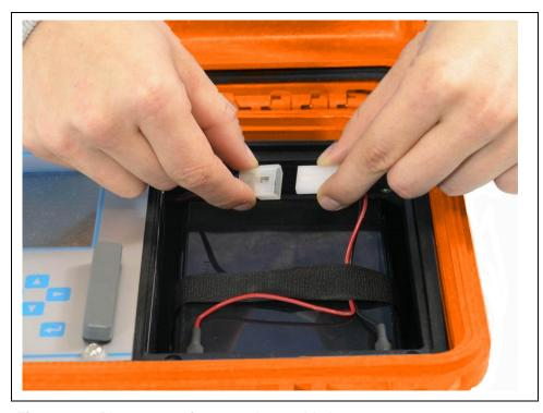
Fig. 6-30 Plug connection to rechargeable battery
