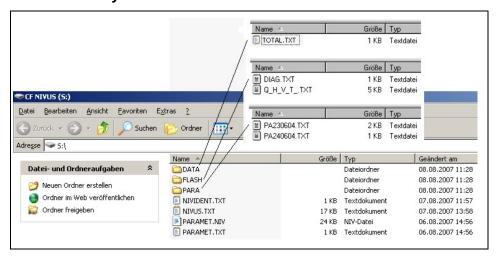
Fig. 8-58 Data structure on memory card
