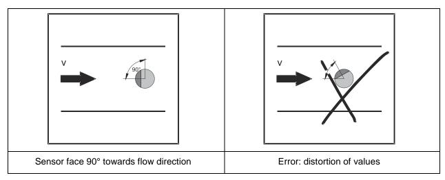
Fig. 6-16 Hints on pipe sensor installation
