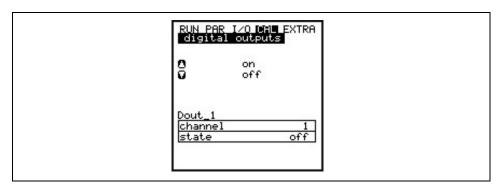
Fig. 8-87 Relay simulation
