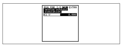
Fig. 8-86 Entering the output value
