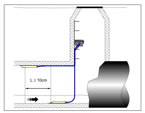
Fig. 6-20 Arranging the sensors
