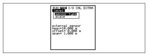
Fig. 8-28 Example screen: external Sensor
