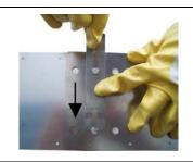
Lock pins by using fastening clip (must sit flush to mounting plate against flow direction)
