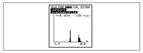
Fig. 8-66 Selecting level measurement echo profile
