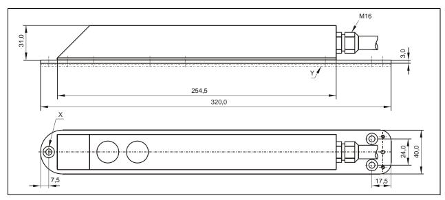
X Countersunk holes according to DIN 74 - A m 5 for direct fastening YThree adapter plates are required for fastening on pipe mounting system
