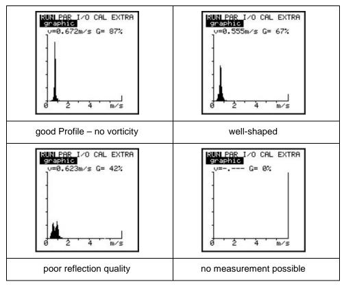
Fig. 8-4 Flow velocity profiles
