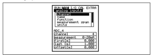
Fig. 8-34 Submenu analog inputs
