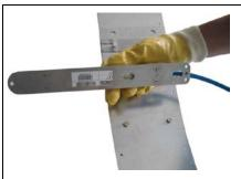
Put the sensor with the cut-outs (slotted holes) onto the plate
