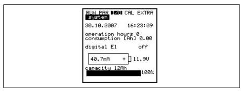
Fig. 8-76 Battery lifetime screen
