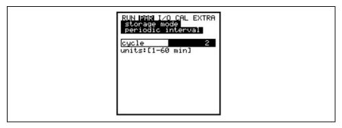
Fig. 8-52 Setting the saving cycle
