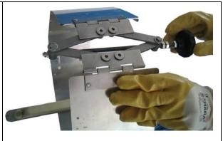
Close the scissors completely by rotating the clamp handle before installing in the channel
