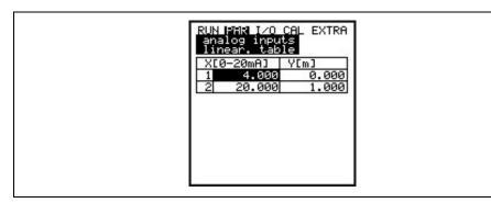
Fig. 8-36 Table of values for analog input span
