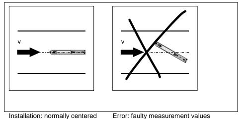
Fig. 6-5 Sensor adjustment
