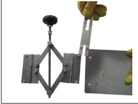
Fix the scissors jack on both sides of the final plate by using the fastening clip
