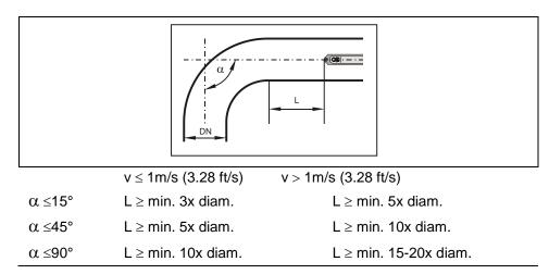
Fig. 6-6 Sensor position behind curves or elbows
