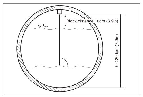
Fig. 6-19 Installation of air-ultrasonic sensor
