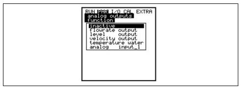
Fig. 8-39 Selecting analog output functions
