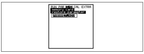
Fig. 8-72 Loading parameters from memory card
