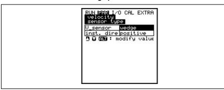
Fig. 8-33 Selecting the sensor type
