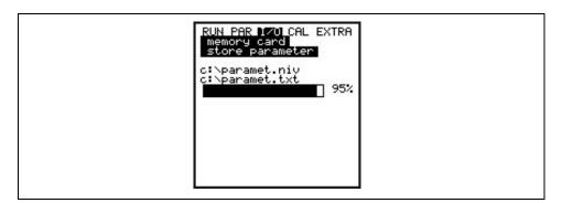
Fig. 8-71 Saving parameters on memory card
