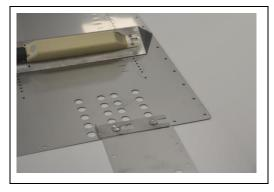
Insert the spigots of the RMS 5 extension sheet into the holes of the base plate and fix the sheet with a clamp.
