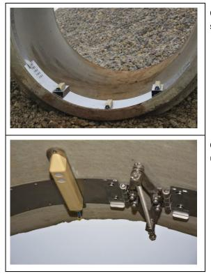
Clamping sheets installed with CS2 sensors
