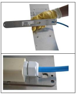
Put the flow velocity sensor onto the base plate with the slotted holes down.
