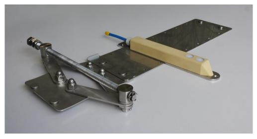
Fig. 7-8 Pre-installed air-ultrasonic sensor on RMS sheet
