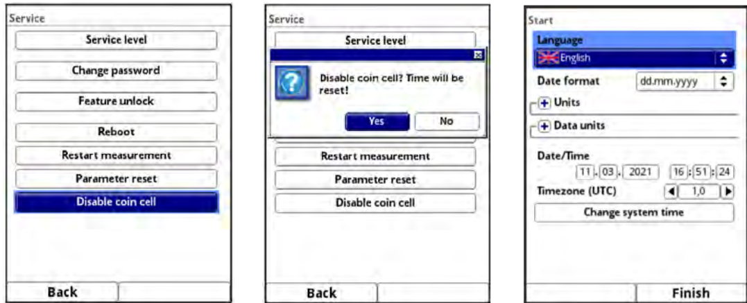
Fig. 36-13 Disable Coin Cell / Putting the Transmitter back into Operation
