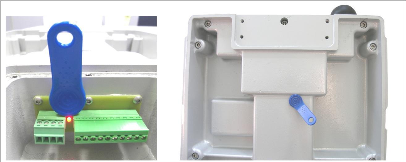
The magnetic switch is activated by passing the delivered magnet over the switch until the status LED flashes 3 times. Then remove the magnet.
