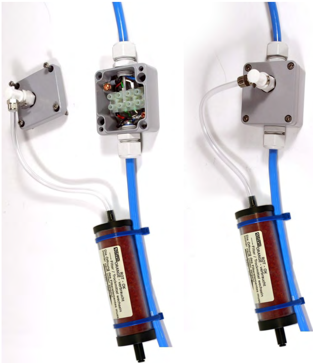
Fig. 5-15 Assembled pressure compensation element
