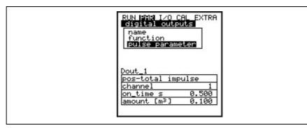
Fig. 7-4 Setting relay pulse parameters
