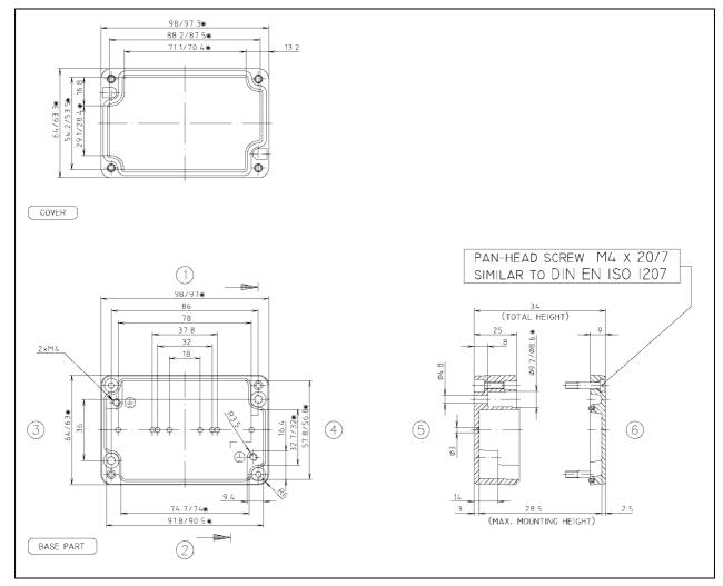
Fig. 6-1 Enclosure sampler terminal box
