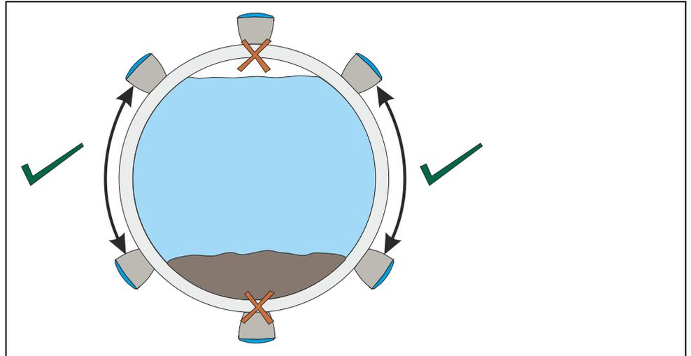
**Fig. 5-1 Recommended positioning on horizontal pipes**
