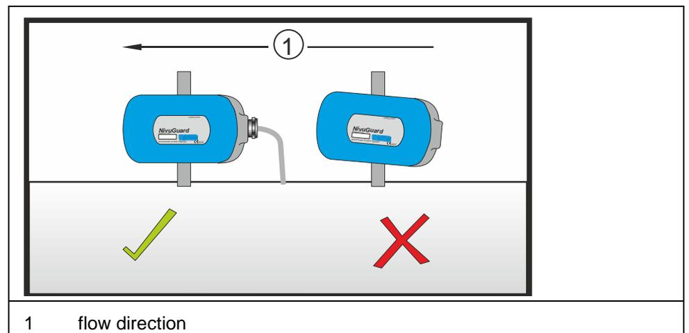
**Fig. 5-2 Sensor correctly aligned along the pipe axis**
