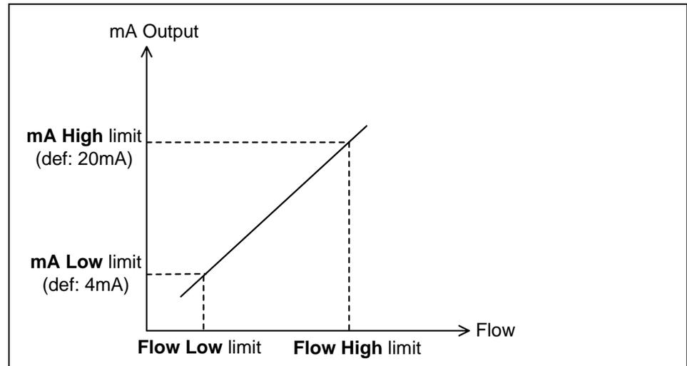
**Fig. 6-5 mA output scaling versus the low-high range of flow**
