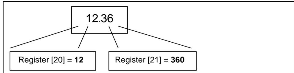
**Fig. 7-1** flow rate format
