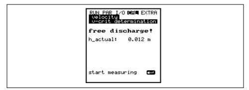
Fig. 8-131 Assistant – start measuring v-crit determination
