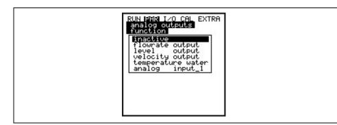
Fig. 8-64 Selecting analog output functions
