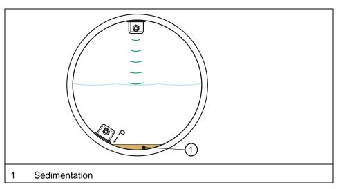
installed out of the channel centre due to heavy sedimentation (Fig. 8-49).
