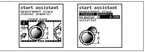
Fig. 8-8 Channel shape and channel geometry selection
