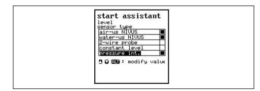
Fig. 8-9 Select level sensor type
