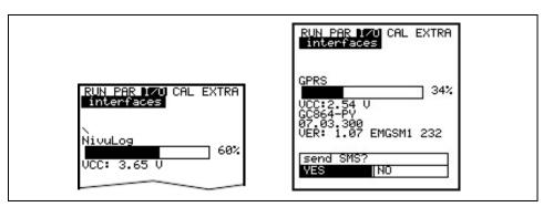
Fig. 8-108 Signal quality screen NivuLog PCM and GSM-Module
