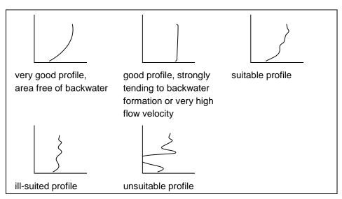
Fig. 8-17 Flow velocity profiles
