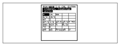
Fig. 8-91 Units of independent readings
