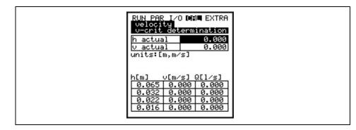
Fig. 8-130 Manually setting v-crit determination
