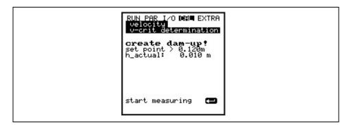
Fig. 8-133 Create dam-up – start measuring
