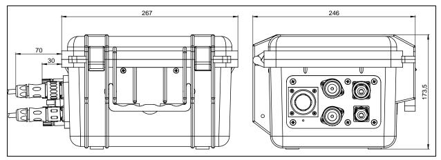
Fig. 6-1 PCM 4 enclosure dimensions and connection sockets
