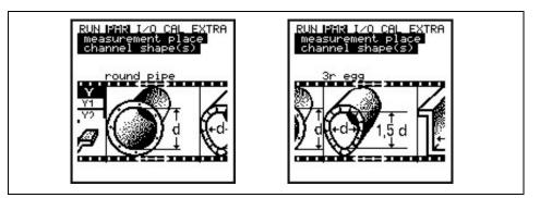
Fig. 8-32 Selecting the channel shape
