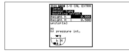
Height h: mounting height "water-US int" + "pressure int." Height H: mounting height "water-US NIVUS"
