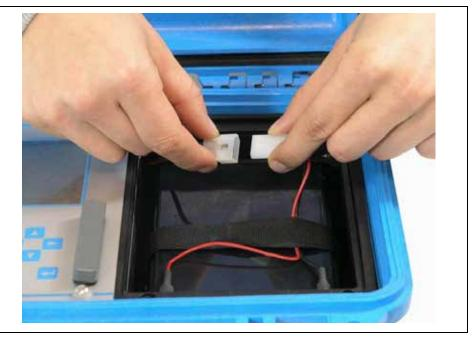
Fig. 6-8 Plug connection to rechargeable battery
