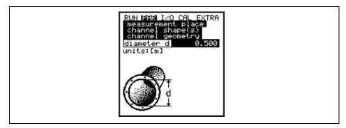
Fig. 8-34 Setting the channel geometry in pipe profiles
