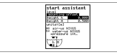
Fig. 8-11 Modifying the mounting offset of level/height sensors
