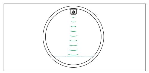
Fig. 8-45 Sensor type 1: Air-Ultrasonic
