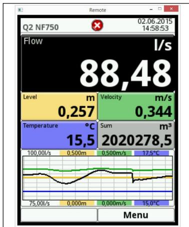
Fig. 8-2 Flow volume section selected
