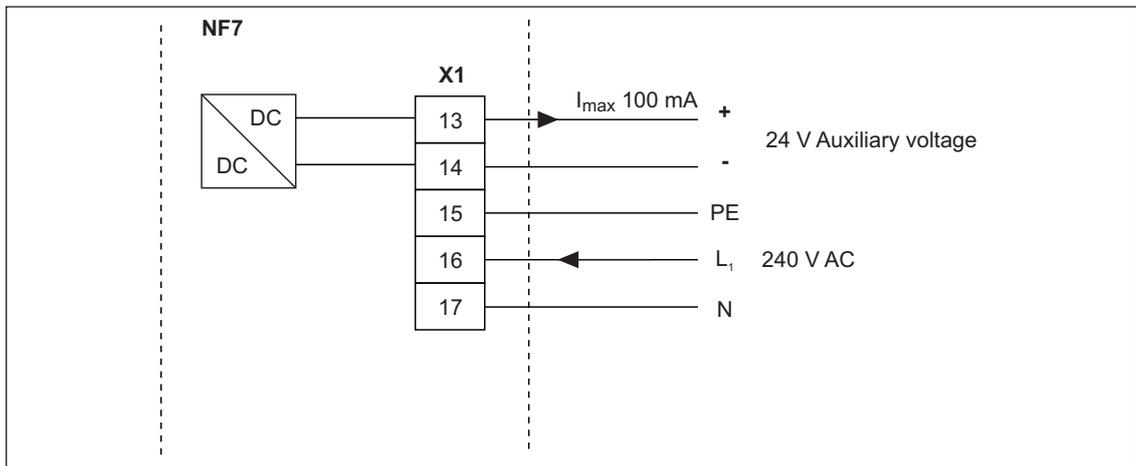
**Fig. 5-28 230 V AC connections of power supply**
