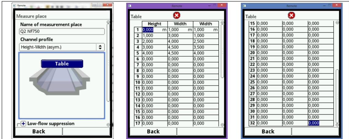
Fig. 7-21 Setting parameters using free asymmetric height-width-width profile
