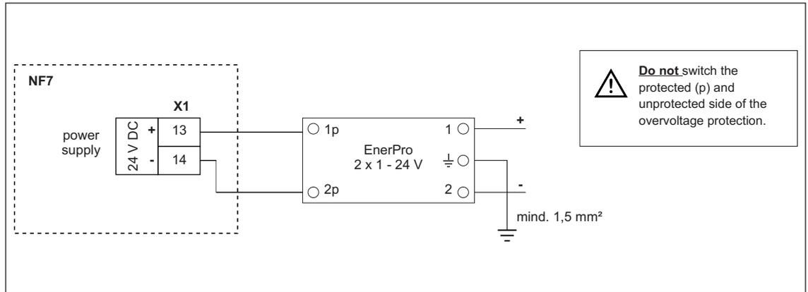
**Fig. 5-16** Overvoltage protection for power supply DC
