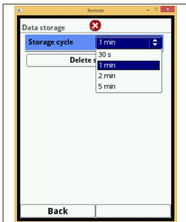
**Fig. 7-133** Setting the storage cycle
