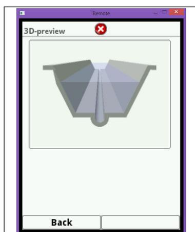
Fig. 7-18 Trapezoid profile with dry weather flume
