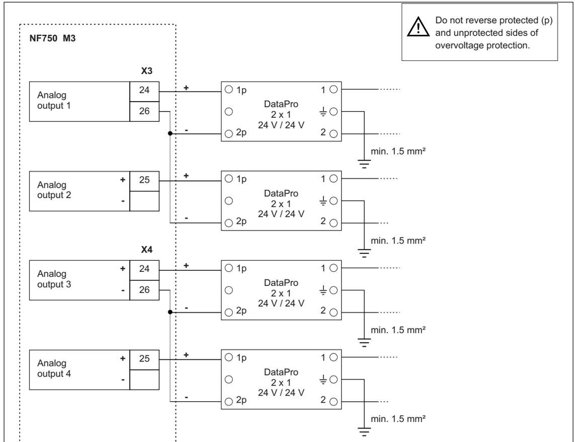
**Fig. 5-22** Overvoltage protection analog outputs NivuFlow 750, type M3
