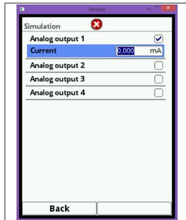
**Fig. 7-97** Setting the desired current value for simulation
