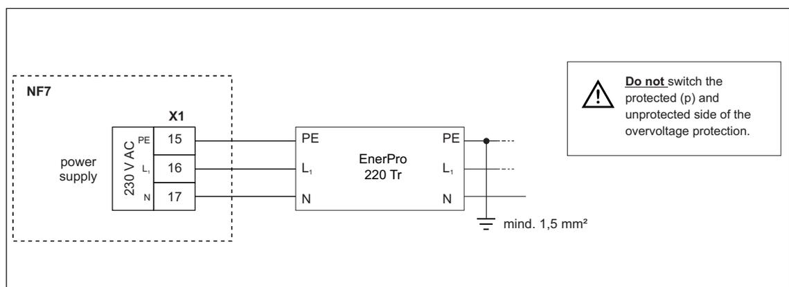
**Fig. 5-15 Overvoltage protection for power supply AC**
