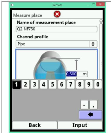
Fig. 7-10 Enter geometry dimensions
