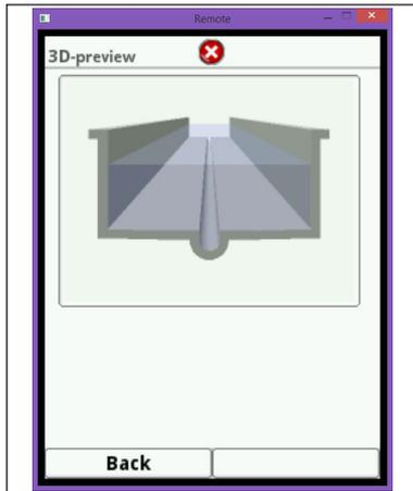
**Fig. 7-19 Trapezoid profile with vertical walls and dry weather flume**
