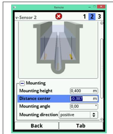
**Fig. 7-44** Entering sensor position, in relation to the application center
