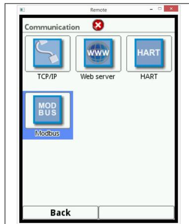
**Fig. 7-161 Modbus programming selection**
