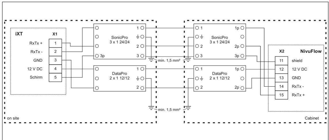
**Fig. 5-23** Overvoltage protection iXT to NivuFlow 750 S1/SR
