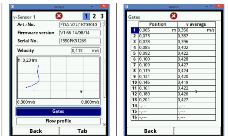
Fig. 8-18 Table of measured individual velocities
