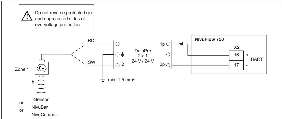
**Fig. 5-20** Overvoltage protection external level measurement
