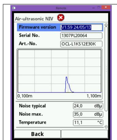
Fig. 7-81 Sensor information and echo image of air-ultrasonic sensor
