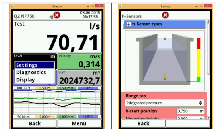
Fig. 8-10 Level sensor settings and their operation ranges
