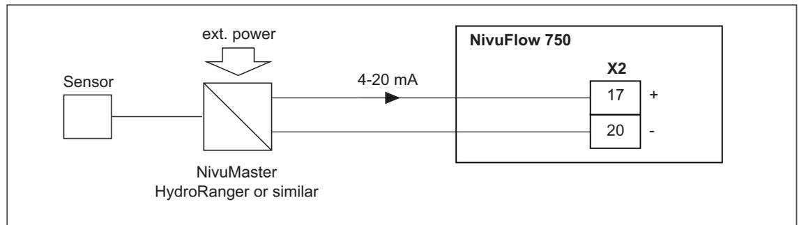
**Fig. 5-14** Connecting an external transmitter
