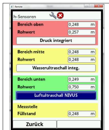
Fig. 7-80 Select air-ultrasonic sensor
