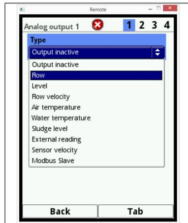
Fig. 7-58 Activation analog output
