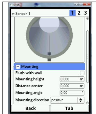
Fig. 7-38 Programming using height, distance and angle
