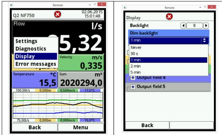
Fig. 8-6 Adjust dimming
