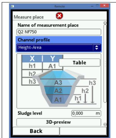
Fig. 7-22 Setting parameters using free asymmetric height-area profile
