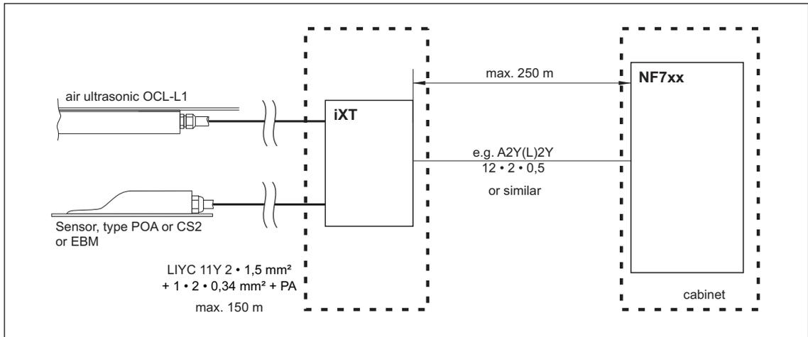
**Fig. 5-8** Connecting iXT to NivuFlow via telecommunications cable
