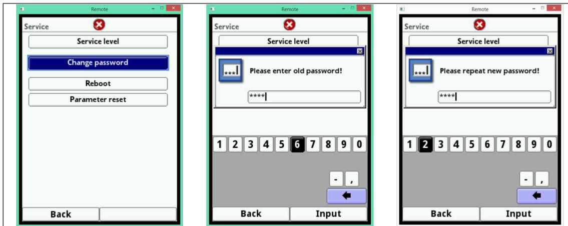
**Fig. 7-154 Changing the password for service level**
