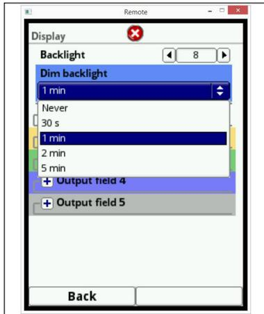
Fig. 7-168 Delay time until backlight dimming
