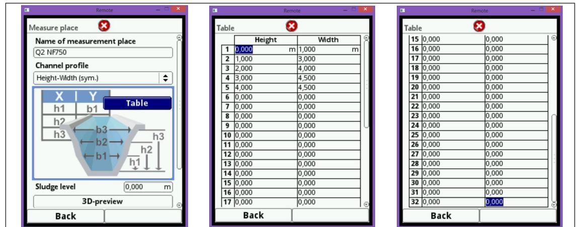
Fig. 7-20 Setting parameters using free symmetric height-width profile
