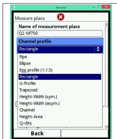
Fig. 7-8 Selectable channel profiles
