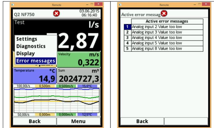
Fig. 8-9 Selection and display of error messages
