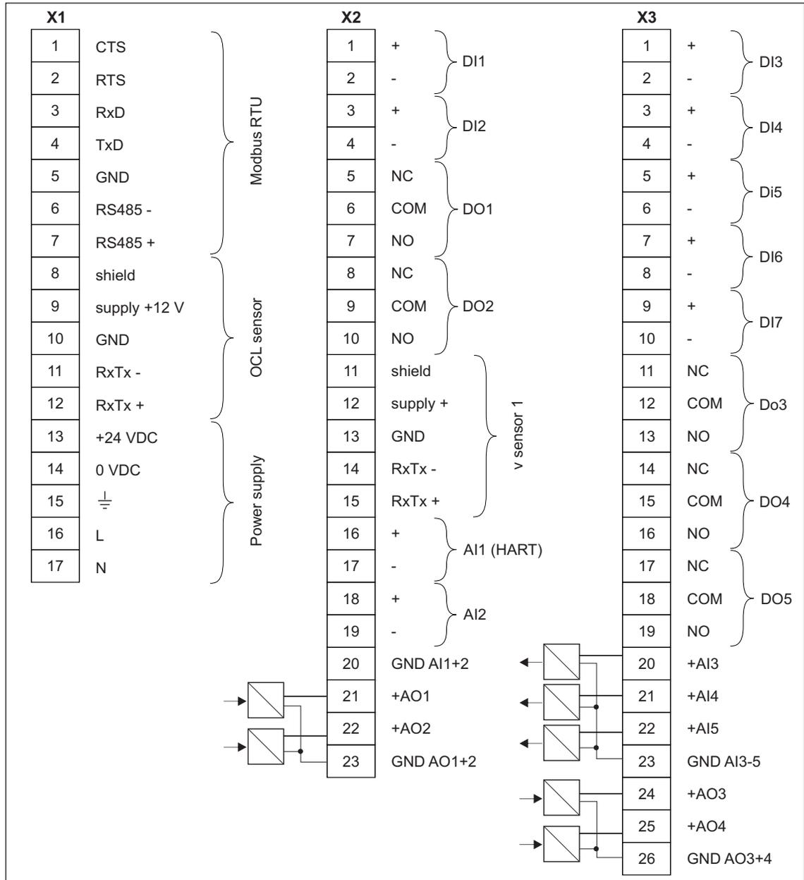
Fig. 5-25 General connection diagram - NivuFlow 750, type SR
