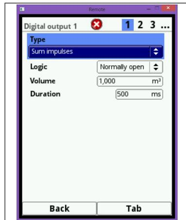
Fig. 7-68 Programming pulse generator
