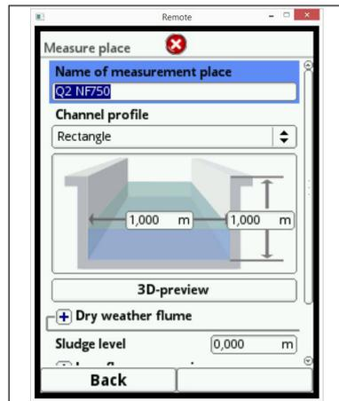
**Fig. 8-4 Measurement place settings**
