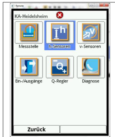
Fig. 7-26 Selection level sensor settings
