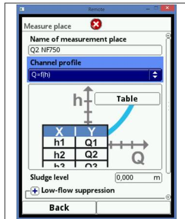
Fig. 7-23 Programming Q/h-characteristics
