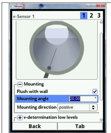
**Fig. 7-40** Flush-mounted display at the right angle
