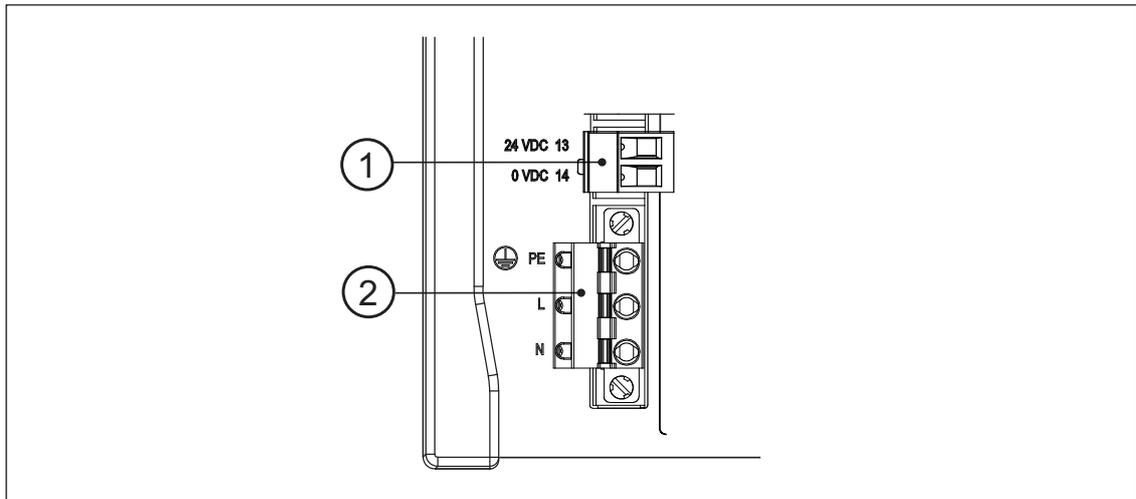
1. 24 VDC connection of type NivuFlow 750
