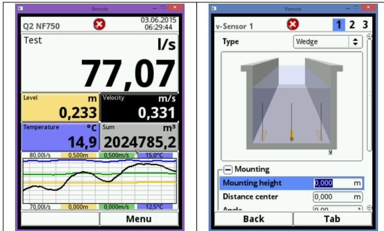
Fig. 8-16 Settings and positions of flow velocity sensors
