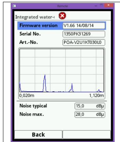
Fig. 7-79 Sensor information and echo image of water-ultrasonic sensor
