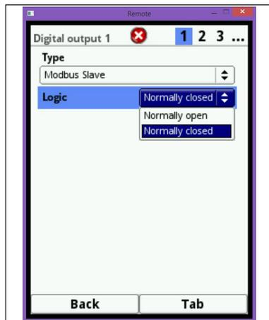
Fig. 7-71 Adjustment options Logic
