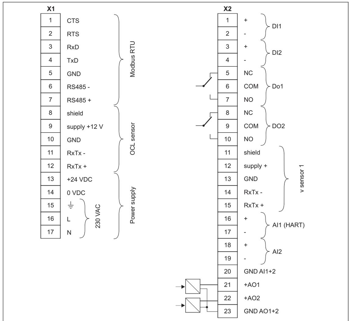
**Fig. 5-24 General connection diagram - NivuFlow 750, type S1**
