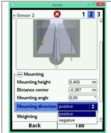
Fig. 7-45 Modifying the sensor mounting direction
