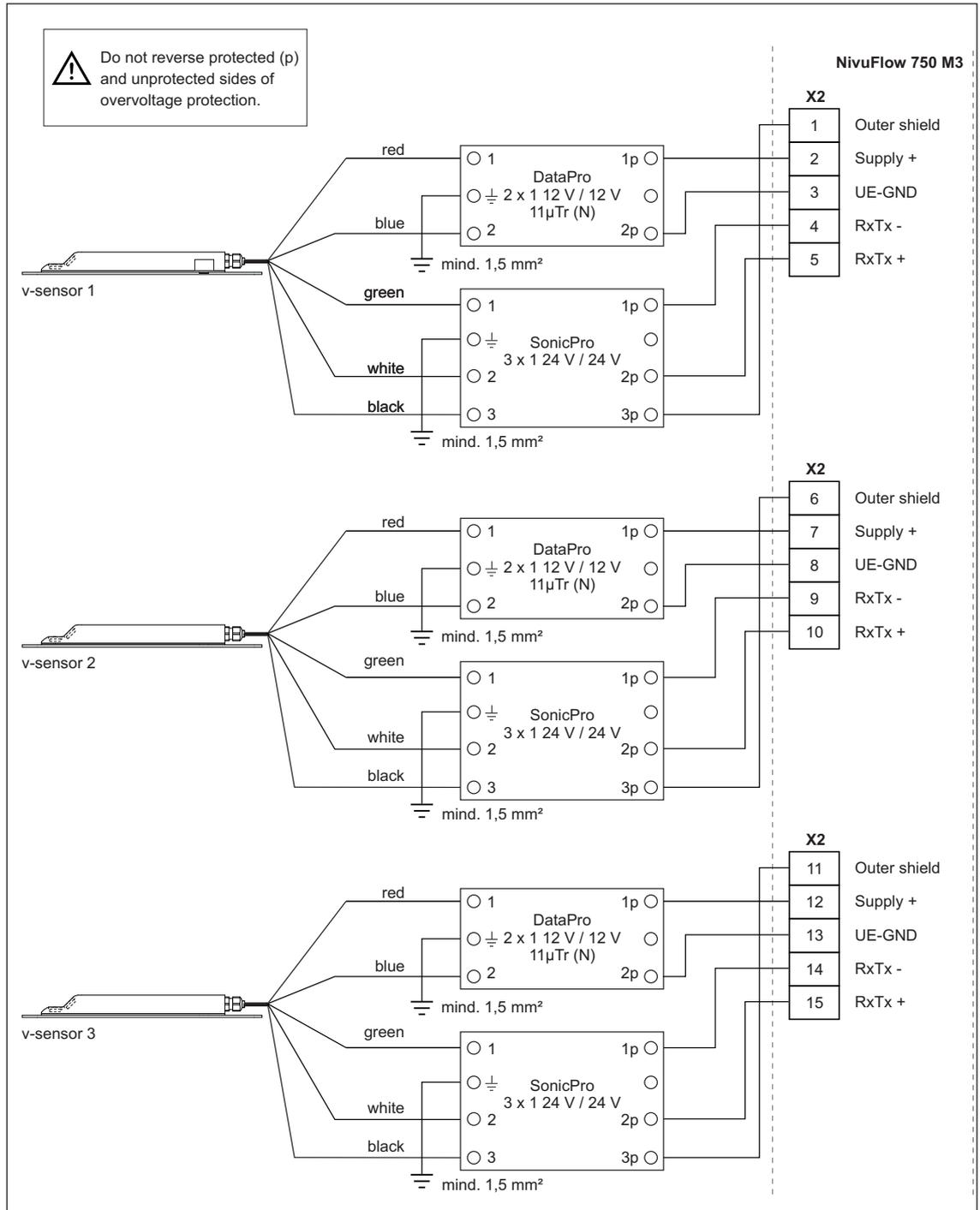
**Fig. 5-19**    **Overvoltage protection Flow velocity sensor to M3**
