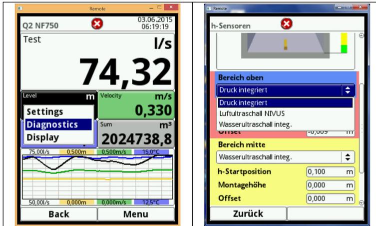
Fig. 8-11 Direct selection of individual sensor diagnostics
