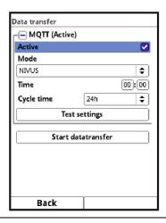
Fig. 10-4 Data Transmission via Network Protocol MQTT
