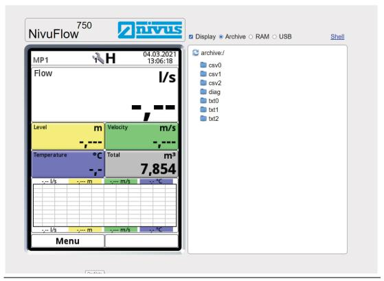
Fig. 9-4 Remote Control via HTTP(S) Web Server
