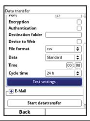
Fig. 10-5 Data Transmission via FTP
