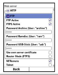
Fig. 9-5 Data Transmission via integrated FTP(S) Web Server
