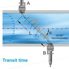
The NivuSonic measurement principle is based on detecting the transit time of ultrasonic signals between two sensors (A and B). The transit time in flow direction  $t_1$  is shorter than it is against the flow direction  $t_2$ . The difference between both transit times is proportional to the average flow velocity along the measurement path  $v_m$ .
