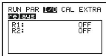
Fig. 30-4 Indication of relay output status
