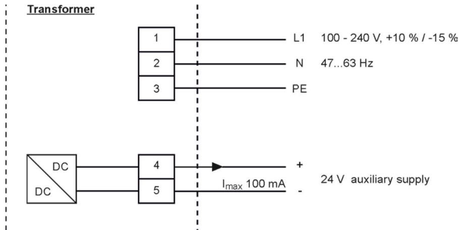
Fig. 20-7 AC model power supply
