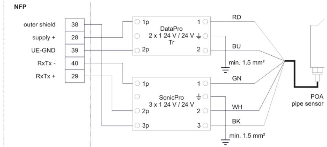
**Fig. 20-11** Connecting the overvoltage protection for velocity sensor Non-Ex version
