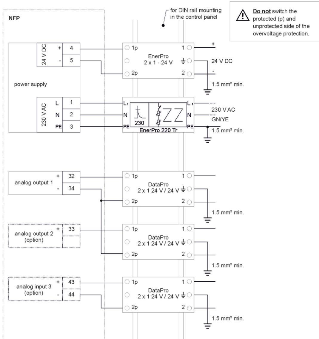
**Fig. 20-9 Connecting the overvoltage protection for power supply and analog outputs**
