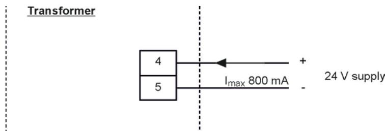
Fig. 20-8 DC model power supply
