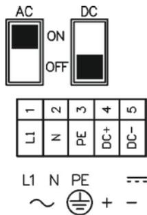
**Fig. 20-6 Slide switch position in terminal clamp housing**
