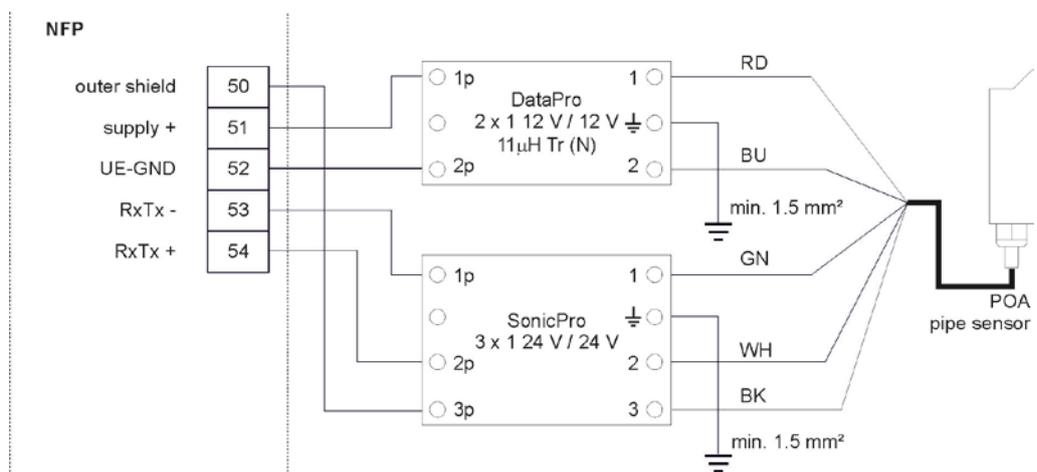
**Fig. 20-10 Connecting the overvoltage protection for velocity sensor Ex version**
