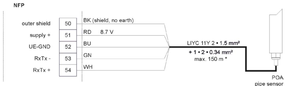
**Fig. 20-4 Connection of a flow velocity sensor Type POA Ex version**
