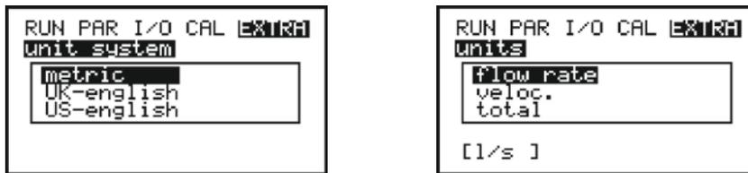
**Fig. 28-3 Selecting the units system and units**
