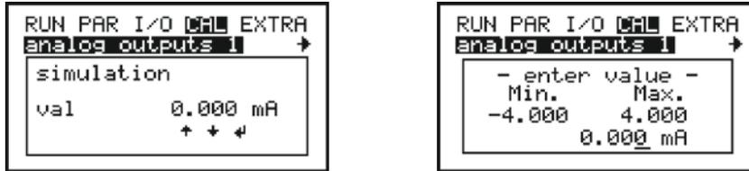
Fig. 31-4 Simulation of analog outputs
