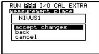
**Fig. 29-4      Accepting the new measurement place name**
