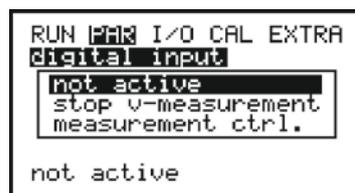
Fig. 29-7 Digital input – function – not active
