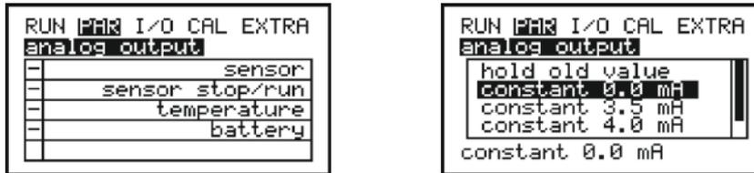
Fig. 29-11 Programming error output
