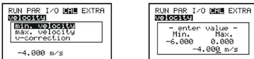
Fig. 31-2 Submenu flow velocity and value settings
