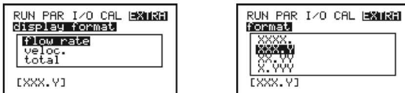
**Fig. 28-4 Selecting the display format**
