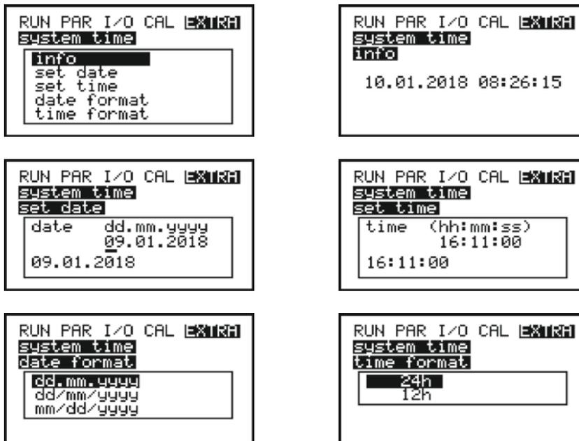
Fig. 28-5 System time submenus
