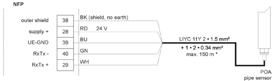
**Fig. 20-5 Connection of a flow velocity sensor Type POA Non-Ex version**
