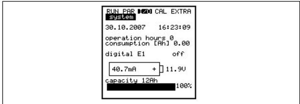
Fig. 8-76 Battery lifetime screen
