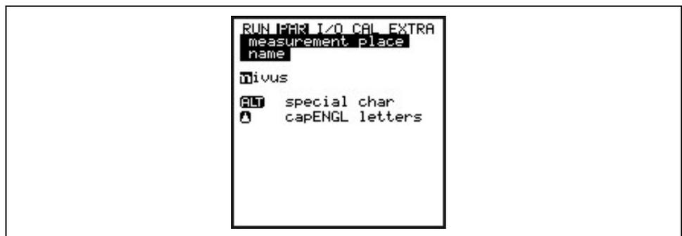
**Fig. 8-19 Setting the name of the measurement place**
