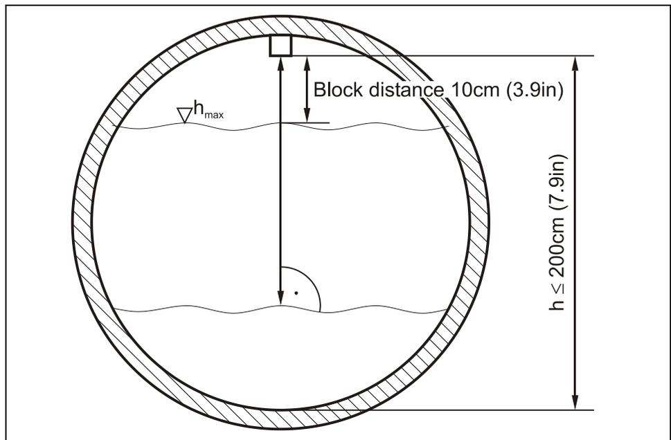
**Fig. 6-19 Installation of air-ultrasonic sensor**
