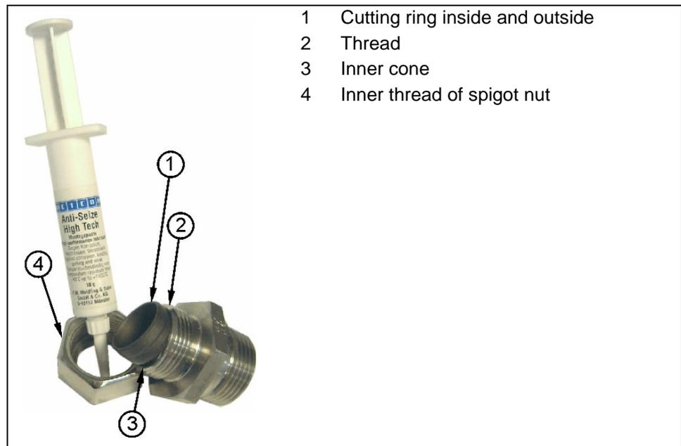
**Fig. 6-17 Using the grease**
