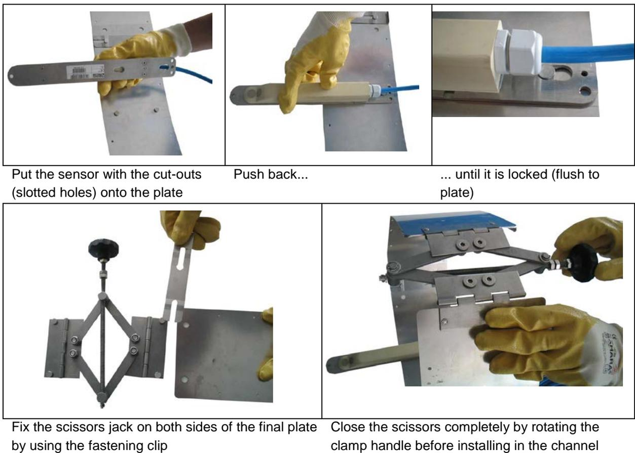
**Fig. 6-23 Assembly of Pipe Mounting System**
