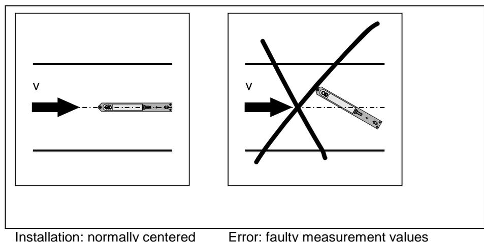
**Fig. 6-5 Sensor adjustment**
