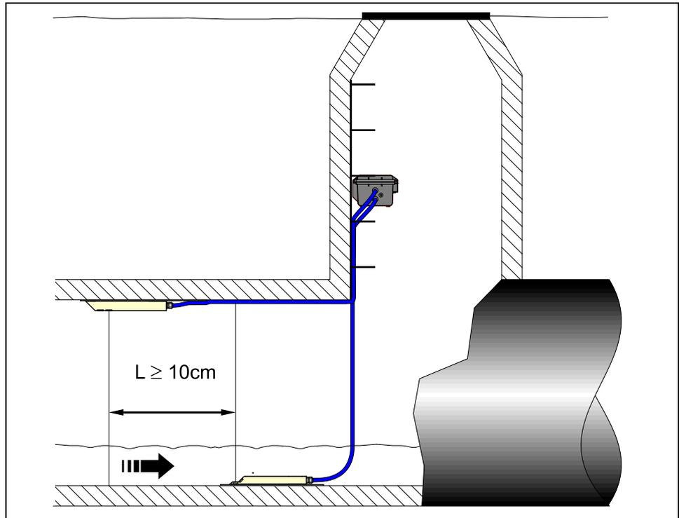
**Fig. 6-20 Arranging the sensors**
