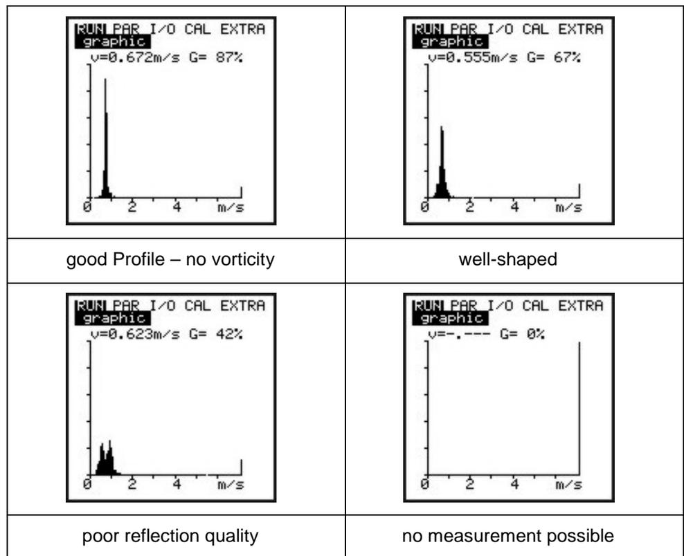
**Fig. 8-4 Flow velocity profiles**
