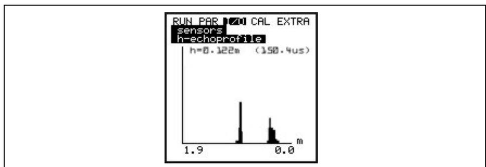
Fig. 8-66 Selecting level measurement echo profile
