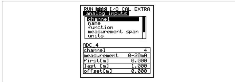
Fig. 8-34 Submenu analog inputs
