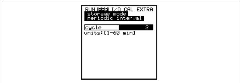
**Fig. 8-52** Setting the saving cycle
