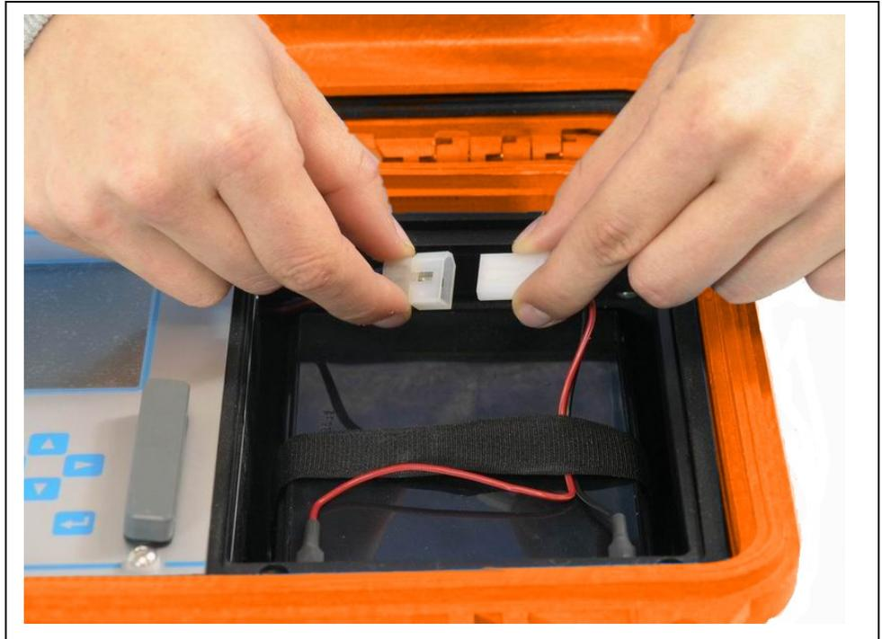
**Fig. 6-30 Plug connection to rechargeable battery**
