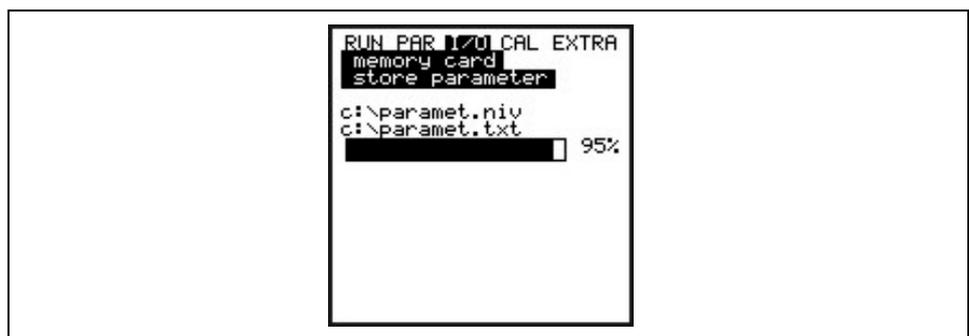
Fig. 8-71 Saving parameters on memory card
