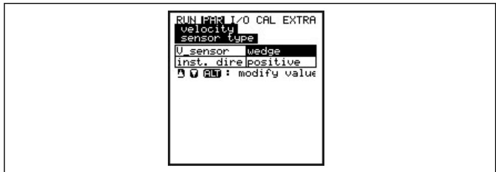
Fig. 8-33 Selecting the sensor type
