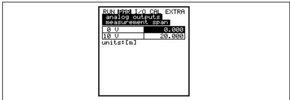
Fig. 8-40 Measurement span
