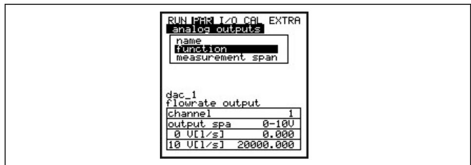
Fig. 8-41 Screen after settings have been made
