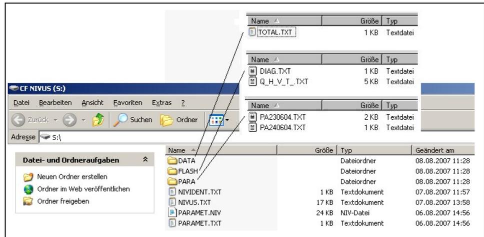
**Fig. 8-58 Data structure on memory card**
