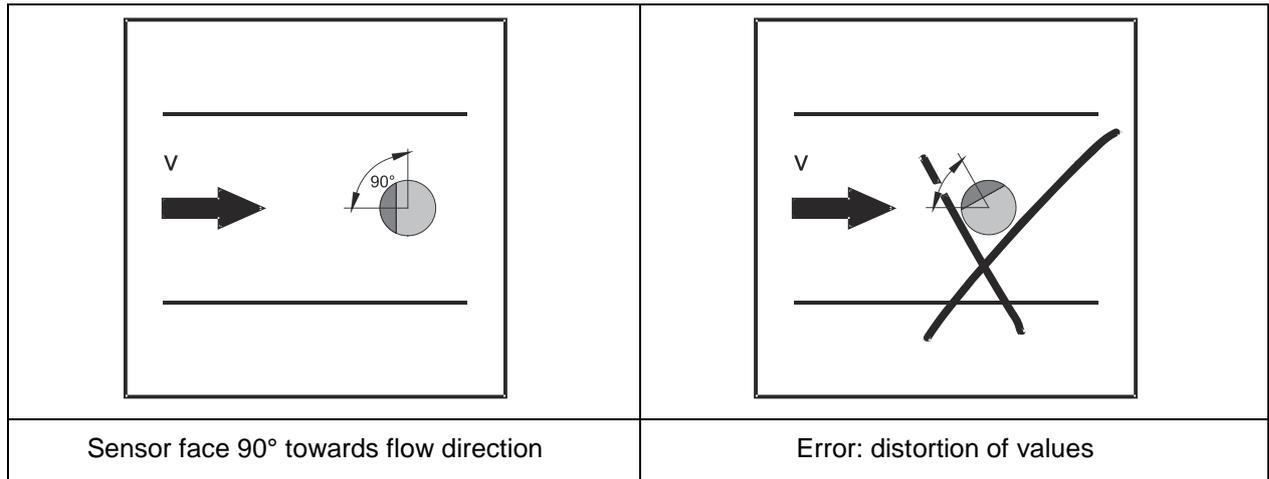
**Fig. 6-16 Hints on pipe sensor installation**
