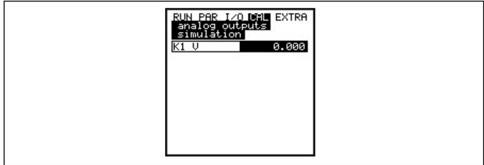
Fig. 8-86 Entering the output value
