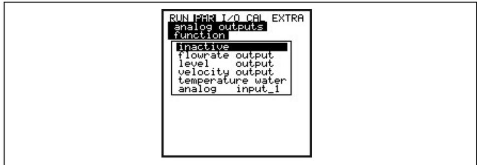
Fig. 8-39 Selecting analog output functions
