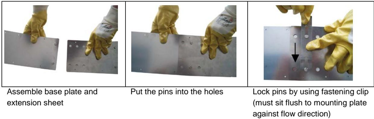
**Fig. 6-22 Installation with fastening clips**
