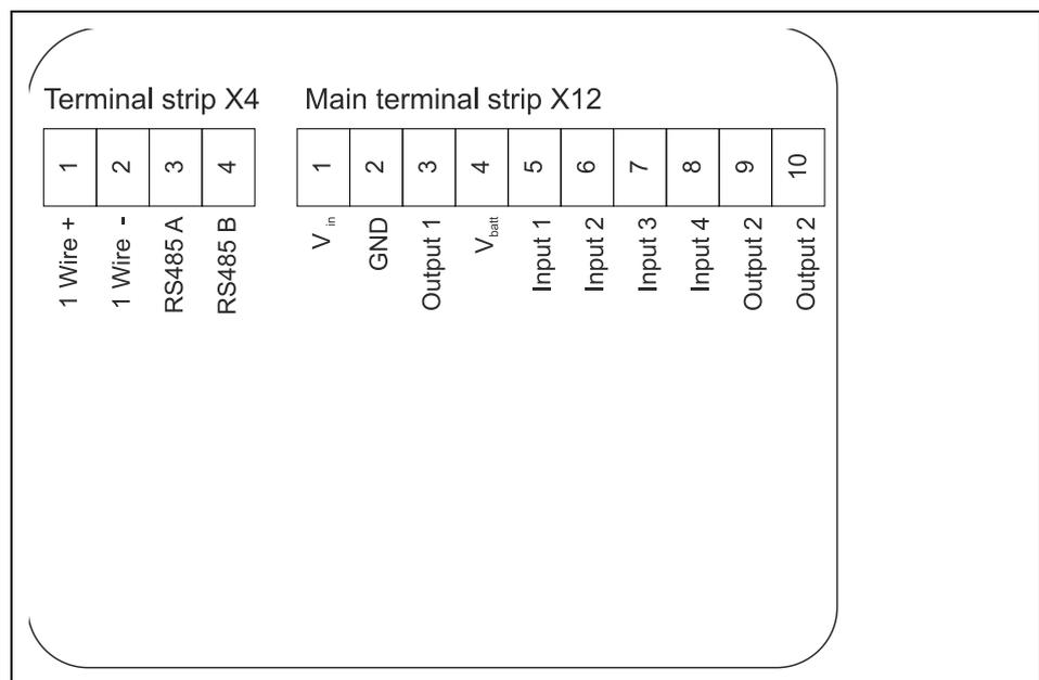
**Fig. 7-2 Connection of sensors and power supply**
