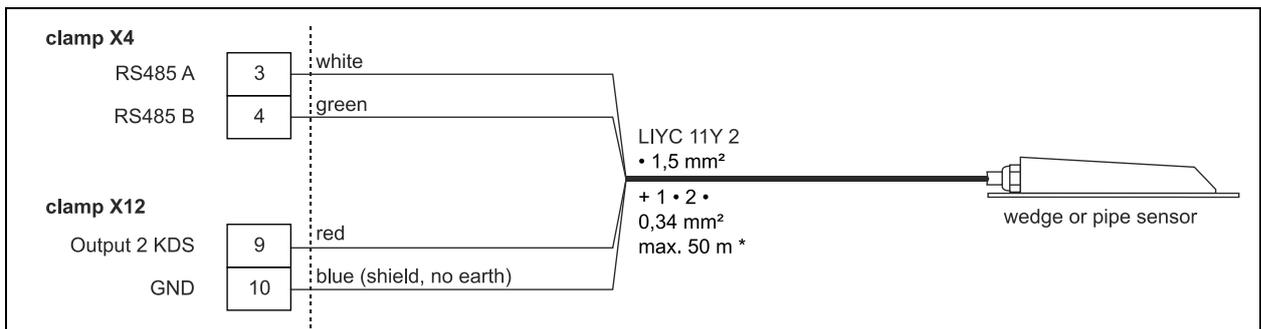
**Fig. 7-4 Connection KDS sensor to NivuLog SunFlow**
