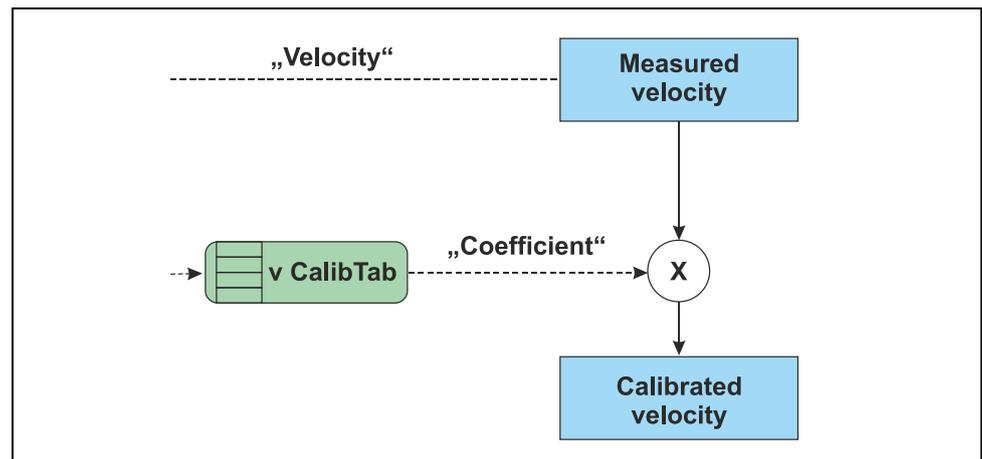
Fig. 9-4 Supplementary explanation to the velocity calibration table
