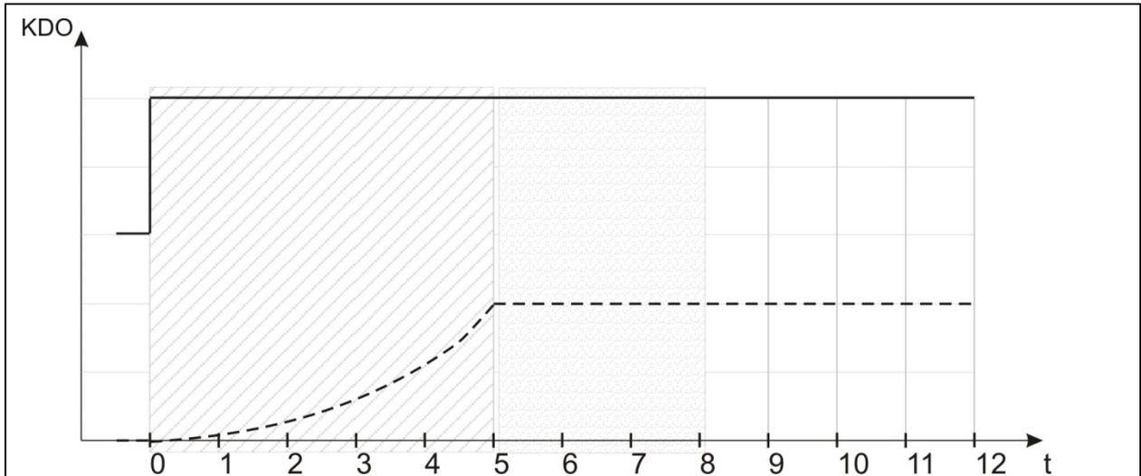
The KDS sensor damps the measurement jump occurring when sensor supply is turned on. Hence a valid reading will not be available before the configurable KDS damping time, which is stored directly in the sensor, has expired. The NivuLog SunFlow does not begin to output readings before the damping time has expired. The "KDS measuring time" directly corresponds with the number of averaged readings since the KDS sensor will output one new reading per second.
