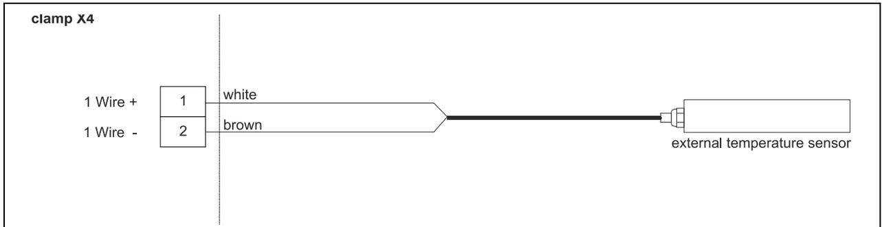
**Fig. 7-3 Connection external temperature sensor to NivuLog SunFlow**
