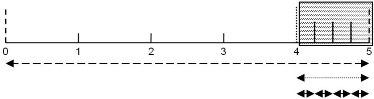
Creation of measurement values: the 4 latest readings are used to create the median and then will be recorded as measurement values.
