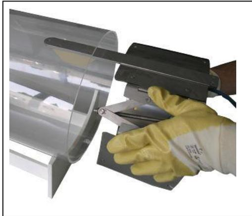
Insert the complete pipe mounting system into the pipe and align accordingly.
