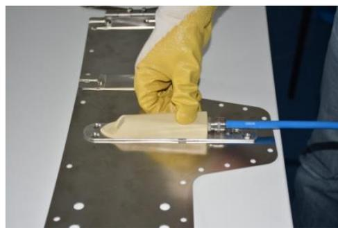
Pull sensor backwards on the completion plate until arrested.
