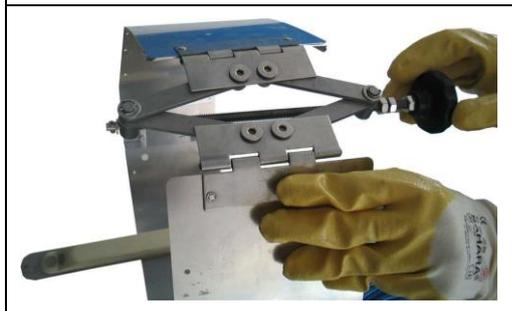
Prior to installation in the channel fully close the clamping device by rotating clockwise.
