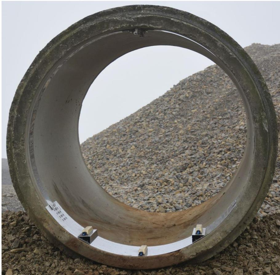
**Fig. 7-7 Clamping device fully assembled**
