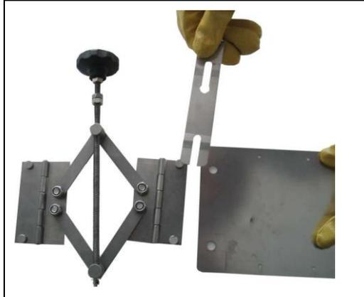
Fasten clamping device to extension sheets on both sides using clamps.
