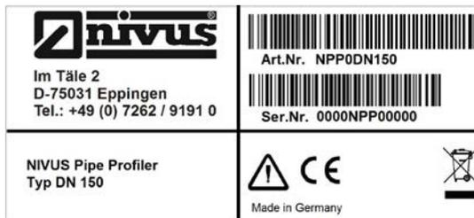
Fig. 4-8 Nameplate NPP0DN...
