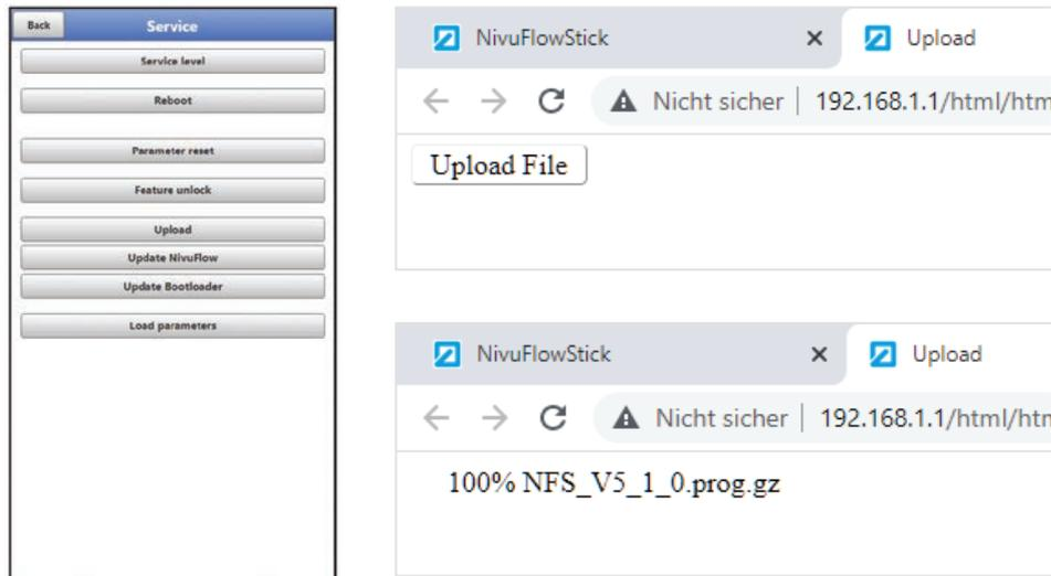
**Fig. 33-12 Upload firmware for NivuFlow Stick update**
