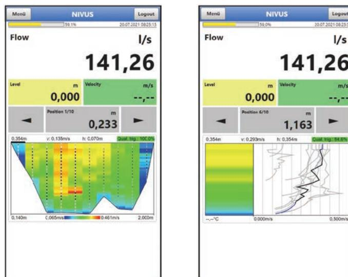
**Fig. 20-4 Measured flow profile**
