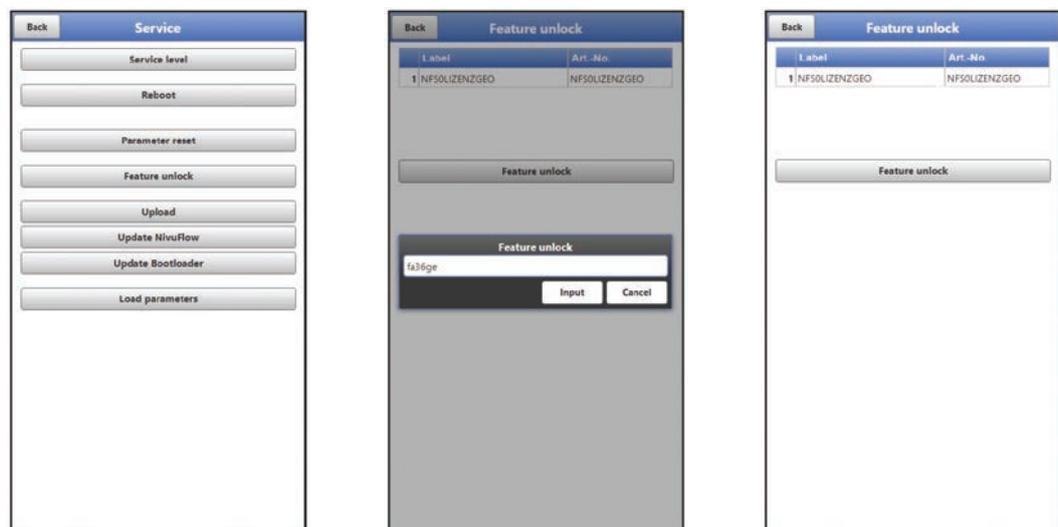
**Fig. 33-8 Activation of the licence in the NFS display tool**
