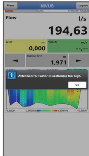
**Fig. 31-13 Message on exceeded flow rate**
