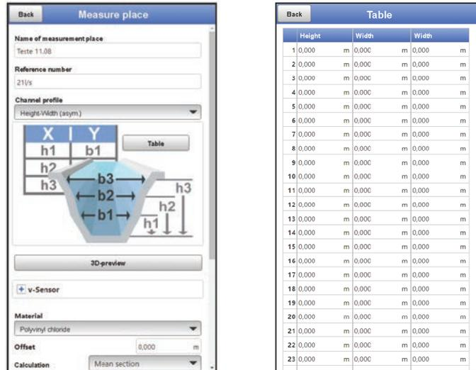
**Fig. 31-5 Asymmetric profile with Height-Width (Height-Width asym.)**
