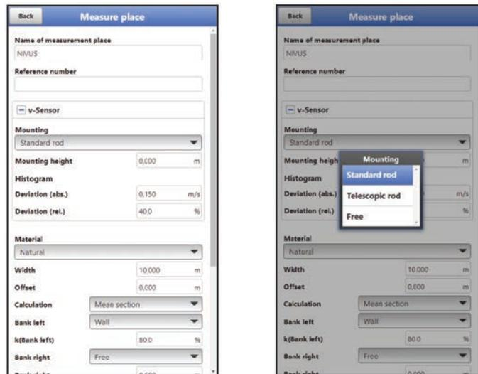
**Fig. 31-6 v-Sensor – Mounting**
