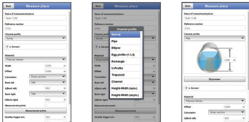
**Fig. 31-3 Channel profile (additional function licence)**
