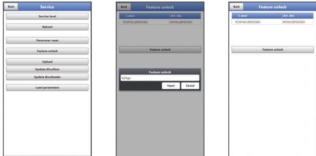
**Fig. 33-10 Activation of the licence in the NFS display tool**
