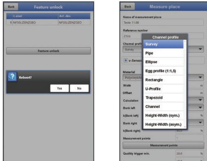
**Fig. 33-9 System reboot after activation / available channel profiles**
