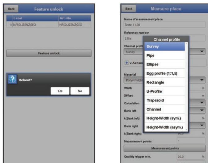
**Fig. 33-11 System reboot after activation / available channel profiles**
