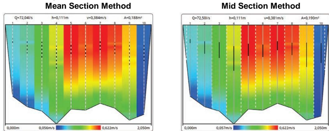
**Fig. 28-11 Representation of the measurement depending on the measurement method (in pdf)**
