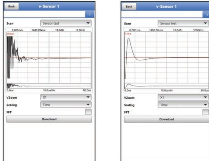
**Fig. 39-3 Signal Analysis Sensor Test / No Sensor detected**
