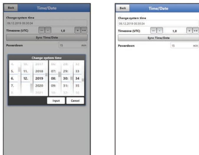
**Fig. 33-4 Change system time: manually and automatically**
