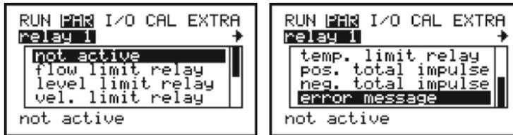
**Fig. 23-28 Relay submenu**
