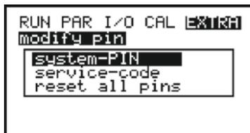
**Fig. 22-7 Submenu modify PIN**
