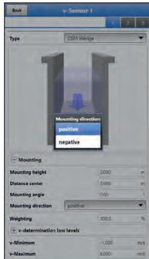
Fig. 39-19 Option to change the Sensor Mounting Direction
