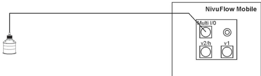
**Fig. 25-3 Connection of i-Series and NivuBar Plus level sensors**
