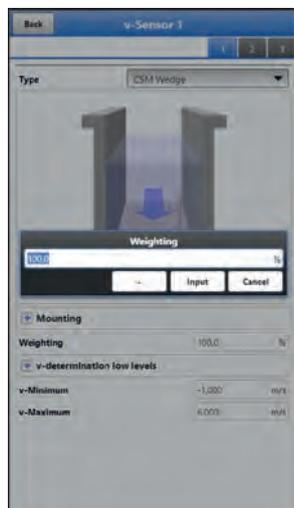
Fig. 39-20 Weighting v-Sensors
