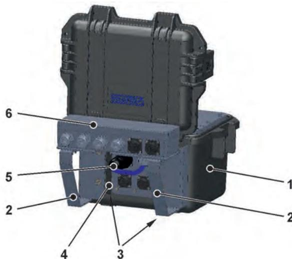
**Fig. 27-1 NFM with Connector Box (principle)**
