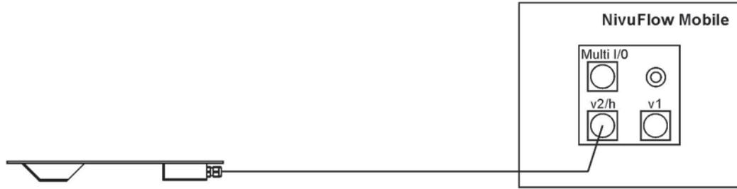
**Fig. 25-2 Connection of DSM-L0 level sensor**
