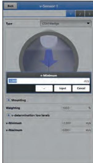
Fig. 39-23 Limiting the Velocity Evaluation
