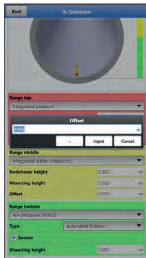
**Fig. 39-12** Setting the parameters of the integrated pressure sensor
