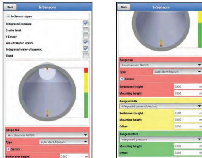
Fig. 39-8 Selecting the Level Sensors
