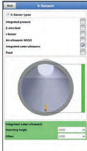
**Fig. 39-7 Selecting the h-Sensor Types**
