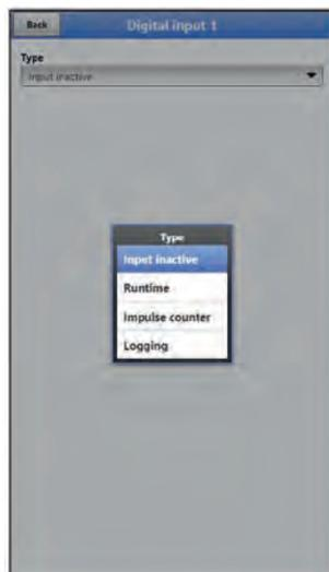
**Fig. 39-27** Activation Digital Input
