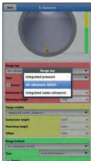
**Fig. 39-11 Assignment Level Sensor to Parameterisation Range**
