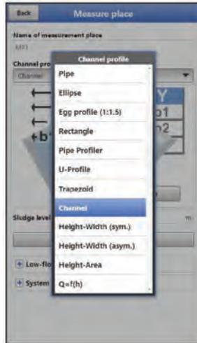
**Fig. 39-2 Selectable Channel Profiles**
