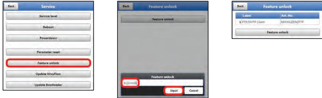
**Fig. 41-9 Activation of the licence in the NFM display tool**
