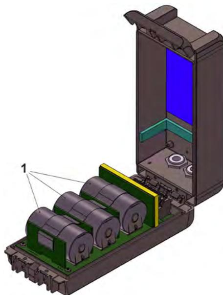
Fig. 2-1 Power supply by batteries
