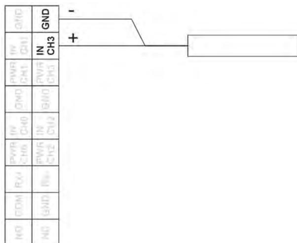
**Fig. 28-4 Connecting an active or passive signal transmitter**
