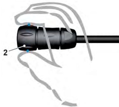
Fig. 25-2 Turning the front ring of the plugs (10-pole/18-pole)
