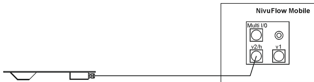
Fig. 26-4 Connection of DSM-L0 level sensor
