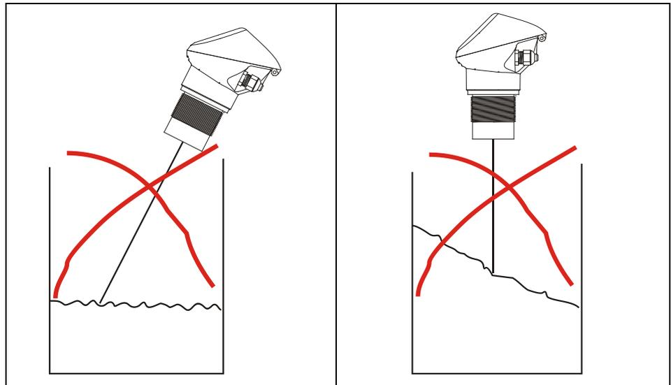
**Fig. 6-12 Incorrect installation of the compact echo sounder**
