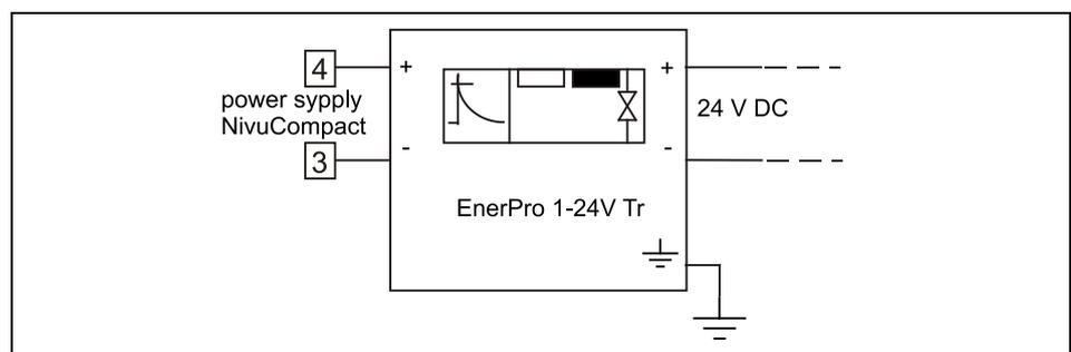
**Fig. 6-10 Overvoltage Protection of operation voltage supply (only 3/4-wire operation)**
