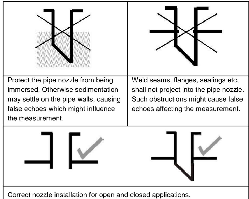
**Fig. 6-15 Installation using a pipe nozzle**
