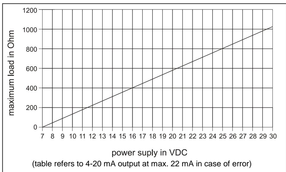
**Fig. 6-4 Maximum load at 3-wire connection**
