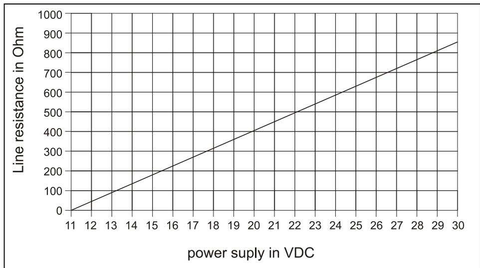
**Fig. 6-3 Maximum permissible line resistance at 2-wire connection**
