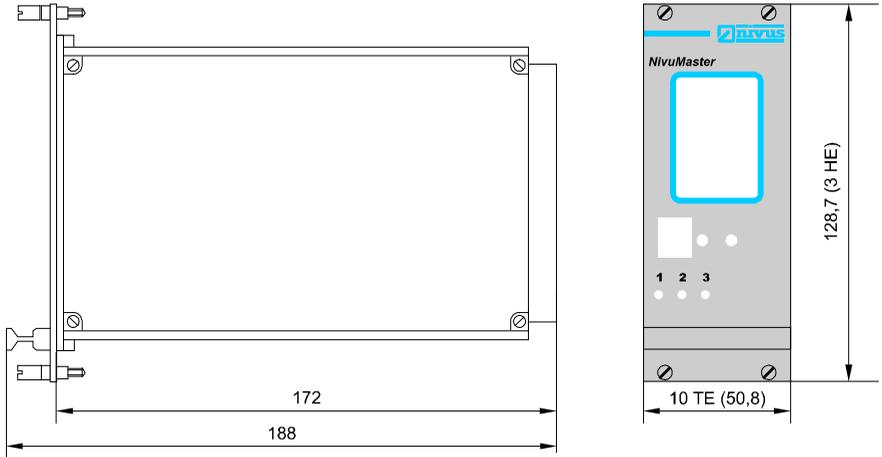
Dimensions of the panel enclosure are as shown below:
