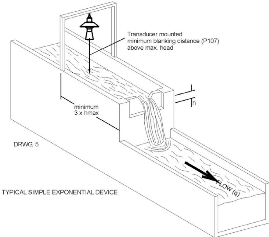
In this example it is required to calculate the flow through a Simple Exponential Device, which on this occasion is a V-Notch Weir. The K factor for the weir is unknown so ratiometric calculation will be used, there is no requirement for alarms and the flow rate is to be displayed in litres/second. The totaliser is to record the flow in cubic metres but is not to be displayed during RUN.
