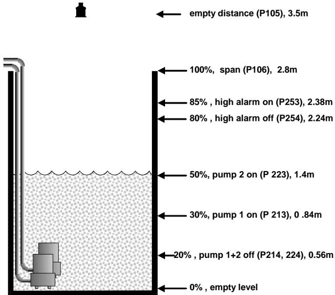
In this example, there are two pumps, which will be set to **alternate duty assist**, so they come on alternately. Pump 1 is to be set to relay 1, pump 2 to relay 2, and the high level alarm to relay 5.
