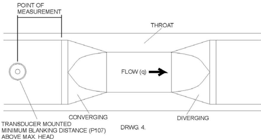
When any **Other** device is chosen please consult the manufacturer of the device for details of where the point of measurement should be located but ensure that it is chosen such that the surface of the liquid is not effected by turbulence or drawdown.
