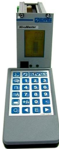
Once communications has been activated, you simply enter the passcode, via the keypad, followed by the ENTER key. The **default passcode** is **1997**, so you would press the following:
