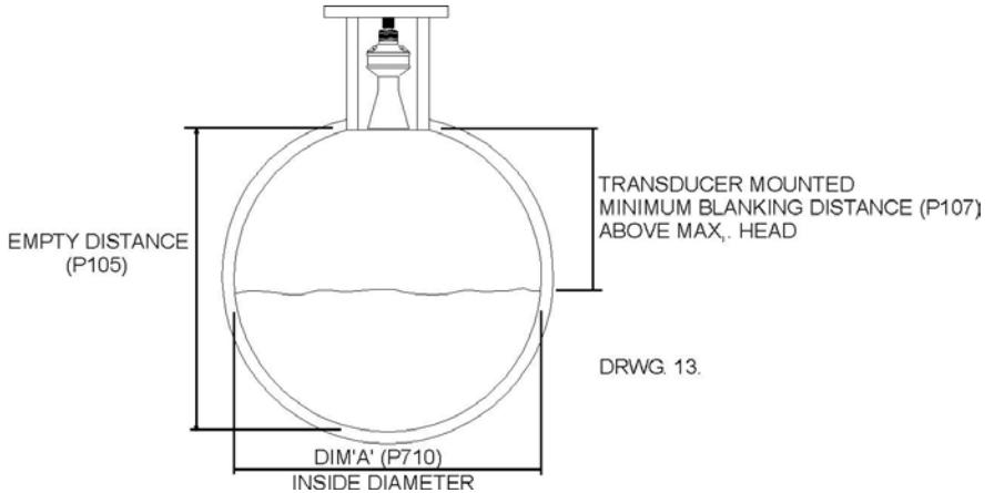
If the flow calculation is to be **absolute P702 = 1** the flow will be calculated using the formula:  $q = va(h)$
