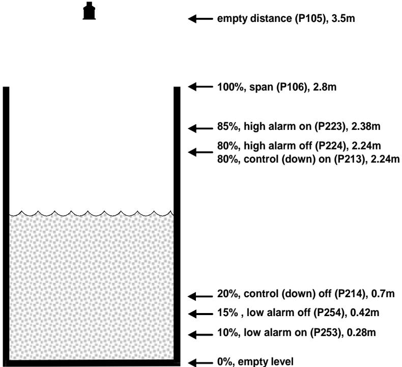
In this example, there is a pump (relay 1), which will come on if the level rises to 2.24 m, and go off when the level drops to 0.7 m. (**control down**). If the level rises to 2.4 m, then the high level alarm (relay 2) will come on until the level drops to 2.24 m. If the level falls to 0.28m, then the low level alarm (relay 5) will come on until the level rises to 0.42 m.
