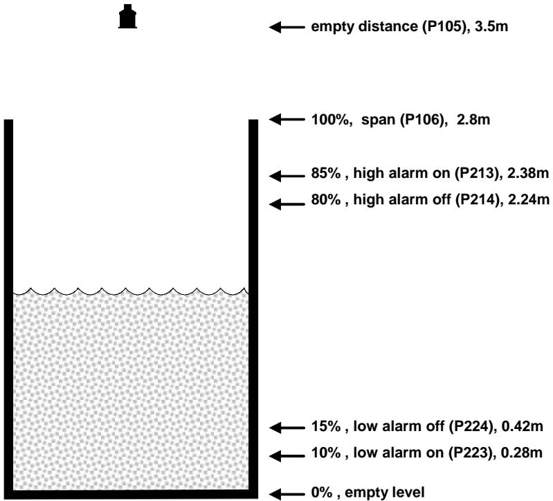
In this example, when the level rises to 2.38 m, relay 1 will come on until the level drops to 2.24 m when it will turn off. If the level drops to 0.28 m, then relay 2 will come on until it rises 0.42 m when it will turn off.
