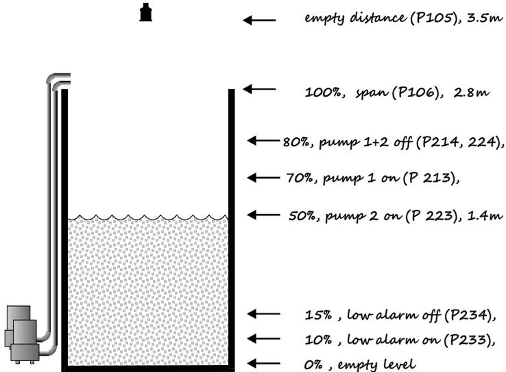
In this example, there are two pumps, which will be set to alternate duty assist, so they come on alternately. Pump 1 is to be set to relay 1, pump 2 to relay 2, and the low level alarm to relay 3.
