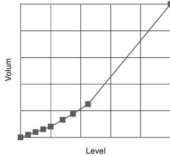
You should enter a level/volume breakpoint for each place where the vessel changes direction, and numerous where the section is slightly curved (mostly linear, but has got a small arc). You can enter any number of pairs between 2 and 32.
