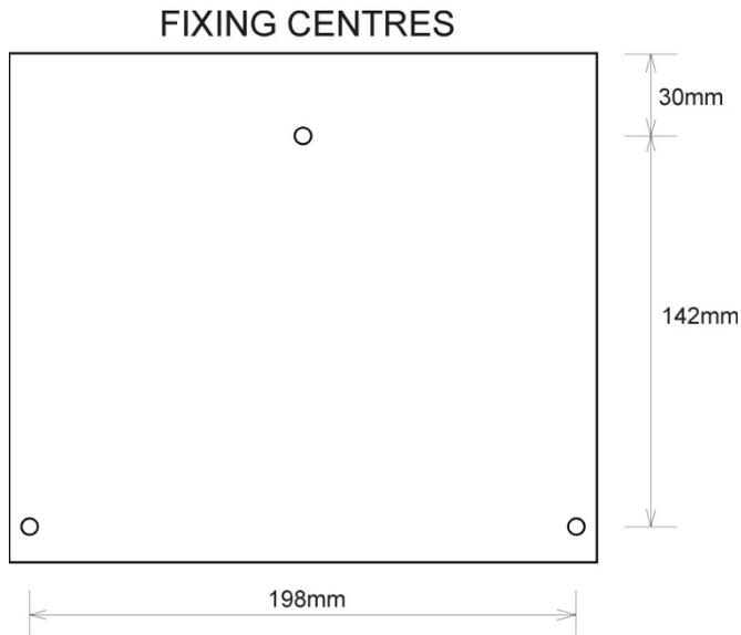
The *NivuMaster* should be mounted by drilling three holes suitable for size 8 screws (length to suit your application), and fixing the top screw in place. Hang the unit on this and fix the two remaining screws by removing the terminals access cover to access the pre drilled holes.
