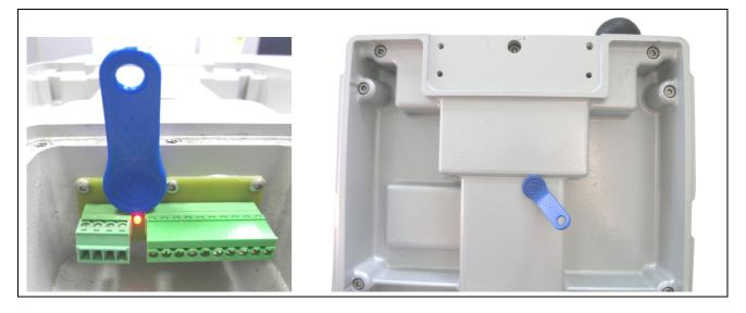
The magnetic switch is activated by passing the delivered magnet over the switch until the status LED flashes 3 times. Then remove the magnet.
