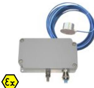
The NDW Inclinometer utilises a capacitive measurement method to measure the inclination (angle measurement) on movable weir flaps. This allows for discharge volume measurement with the aid of the “HydraulicCalculator Plus“ transmitter.
