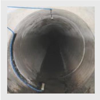
**Flow measurement with cross correlation wedge sensor within a pipe**
