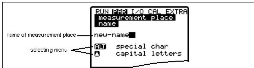
**Fig. 8-15 Setting the name of the measurement place**
