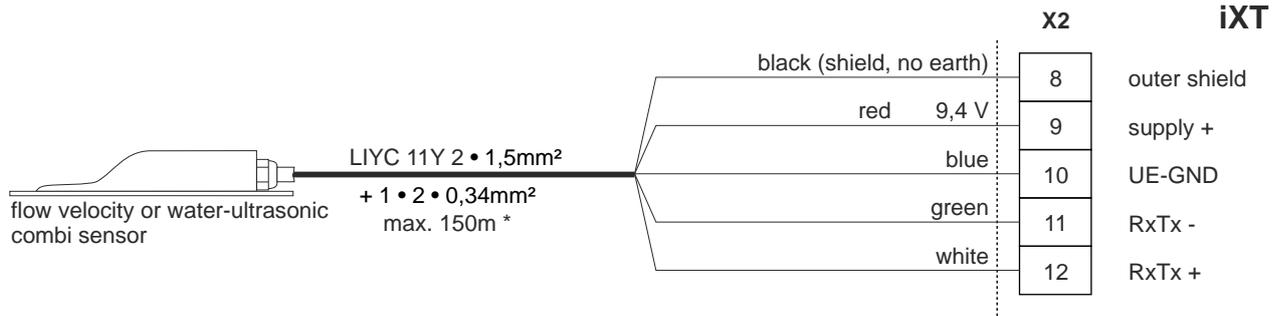
**Connection of the 2. flow velocity sensor to the separation interface type iXT4xx**
