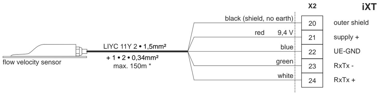
\*Cable extension up to max. 250m (820.3ft) with max. 30m (98.4ft) fixed sensor cable and extension cable with at least A2Y 6 • 2 • 0.8 possible only.
