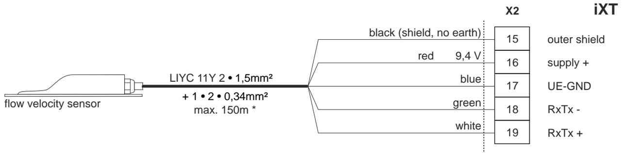
**Connection of the 3. flow velocity sensor to the separation interface type iXT4xx**
