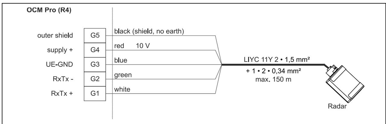
**Fig. 7-10 Connecting an OFR flow velocity sensor to Type R4W0**
