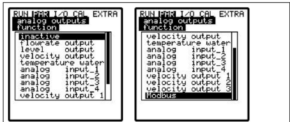
Fig. 9-70 Selection of analog output functions
