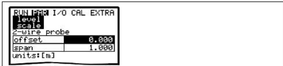
Fig. 9-49 2-wire sensor settings
