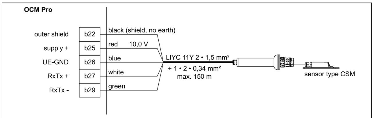
**Fig. 7-25 Connection 2, electronic box Type EBM with water-ultrasonic sensor Type CSM to Type M4F0**
