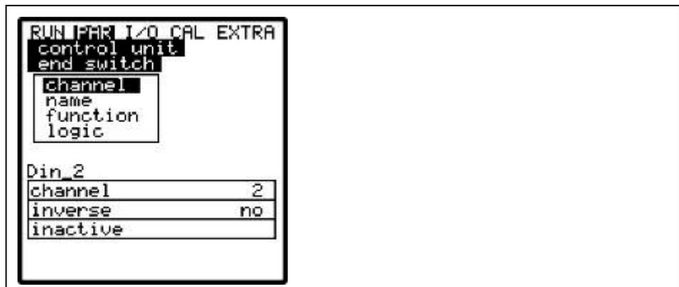
**Fig. 9-80 End switch assignment**
