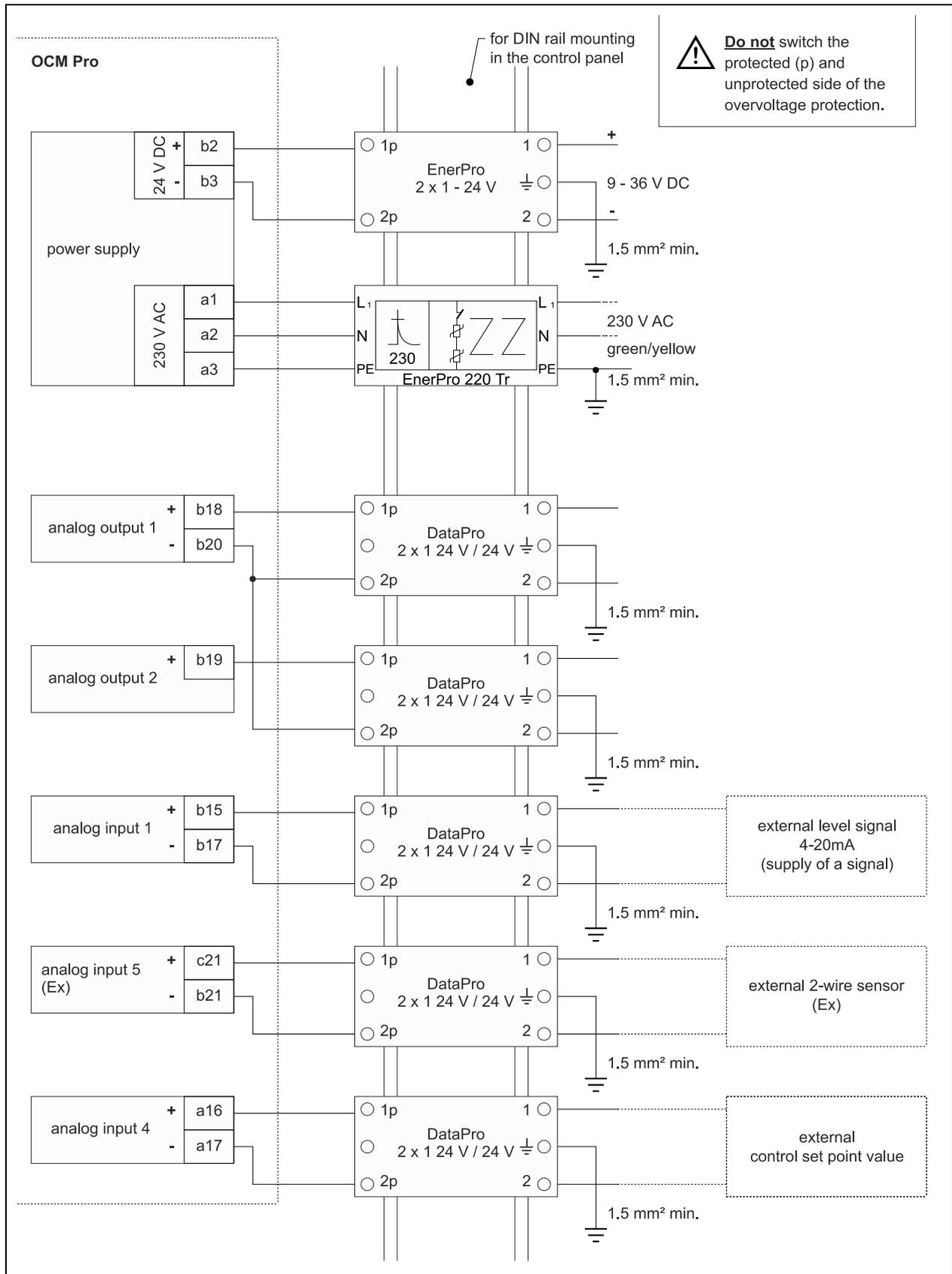
**Fig. 7-32** Panel mount enclosure - connecting the overvoltage protection for power supply and analog inputs and outputs (panel mount enclosure)
