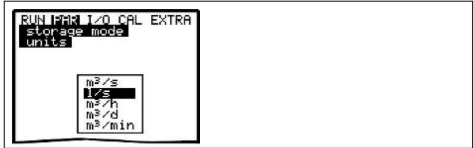
Fig. 9-108 Selecting the units in storage mode
