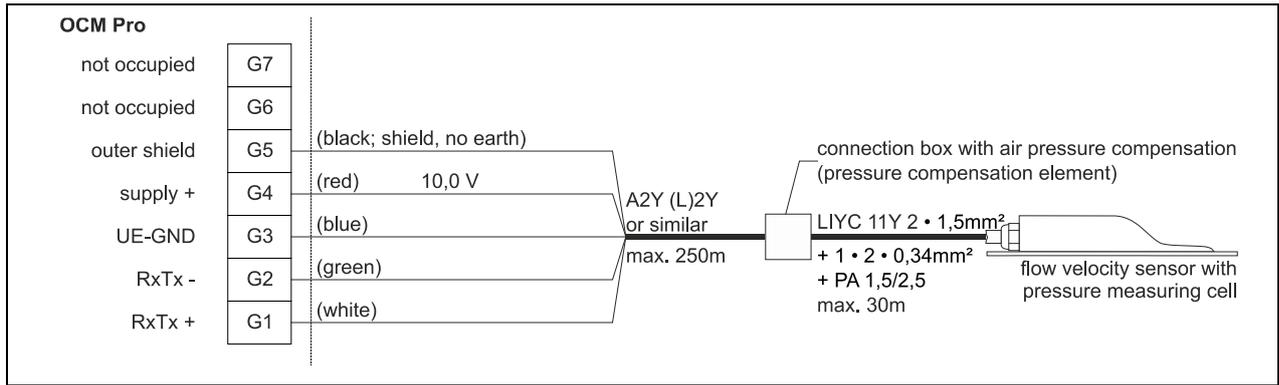
**Fig. 7-9 Connecting a flow velocity sensor with integrated pressure measurement cell to type W0**
