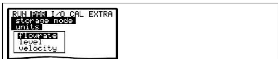
Fig. 9-107 Selecting the measurement value in storage mode
