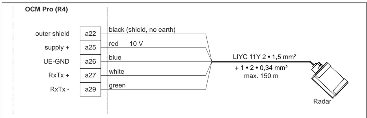
**Fig. 7-21 Connecting an OFR flow velocity sensor to Type R4F0**
