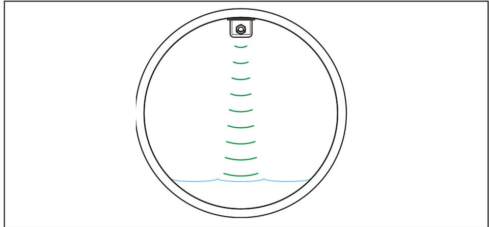
**Fig. 9-33 Sensor type 1: air-ultrasonic**
