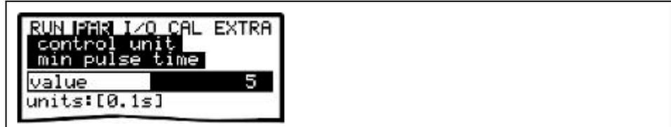
Fig. 9-85 Setting the minimum duration of control impulses
