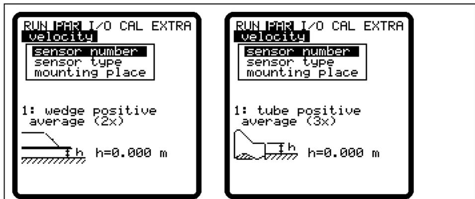
Fig. 9-60 Screen sensor type with 2 or 3 sensors
