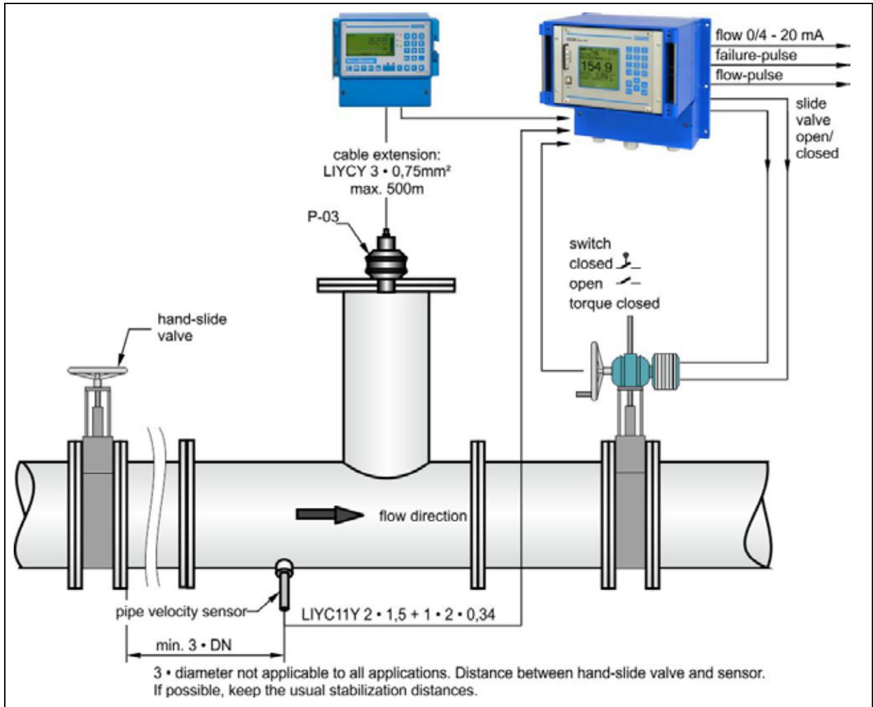
Fig. 7-38 Setup of a controlled system such as a discharge control
