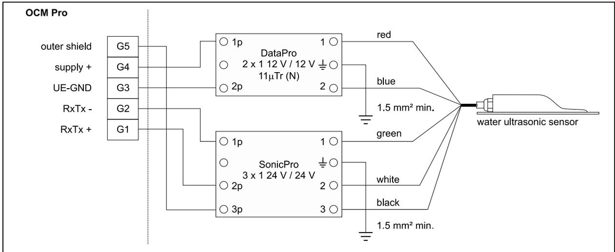
**Fig. 7-16** Overvoltage protection water-ultrasonic sensor or electronic box, wall mount enclosure
