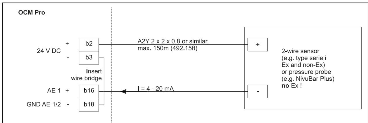
**Fig. 7-13 Connecting a 2-wire sensor for level measurement to type W0**
