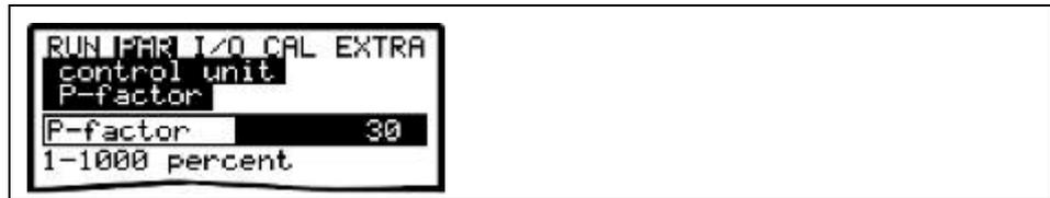
**Fig. 9-82 Assignment of P-Factor**
