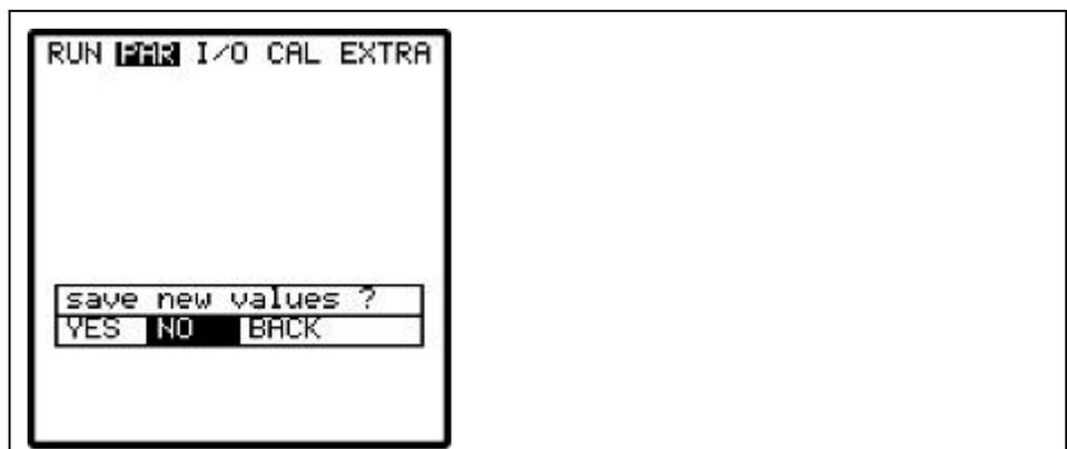
**Fig. 9-1** Screen at end of parameter setting
