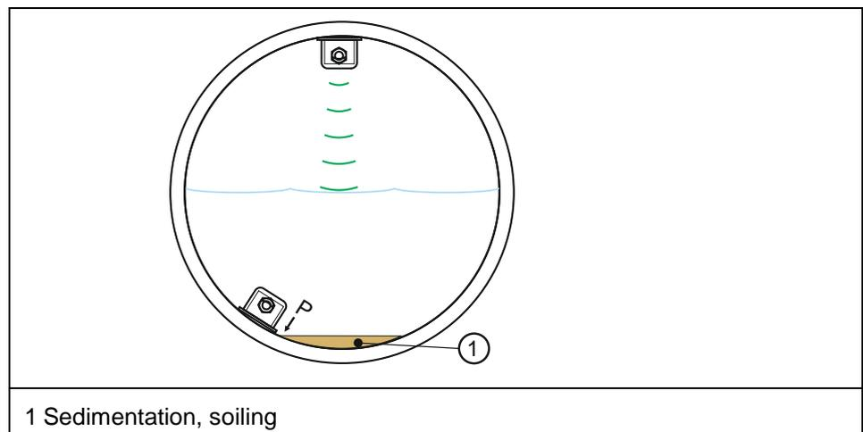
**Fig. 9-39 Combination: Air-ultrasound and internal pressure**
