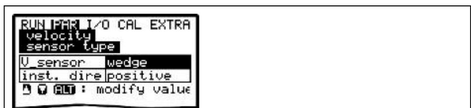
**Fig. 9-53 Select sensor type and mounting position**
