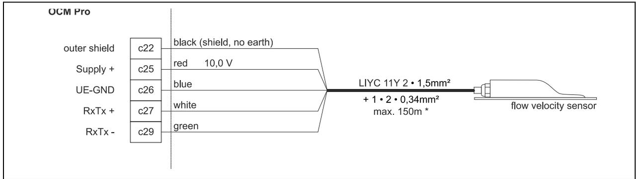
**Fig. 7-23 Connecting a third flow velocity sensor to type M4F0**
