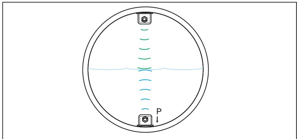
**Fig. 9-41 Air- and water-ultrasound**
