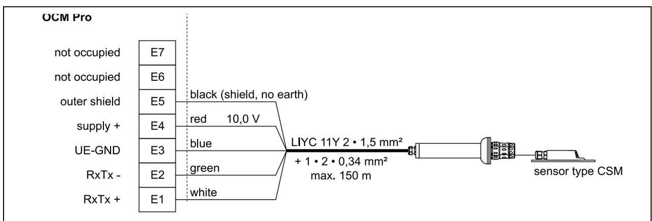
**Fig. 7-8 Connection 3, electronic box Type EBM with water-ultrasonic sensor Type CSM to Type M4W0**
