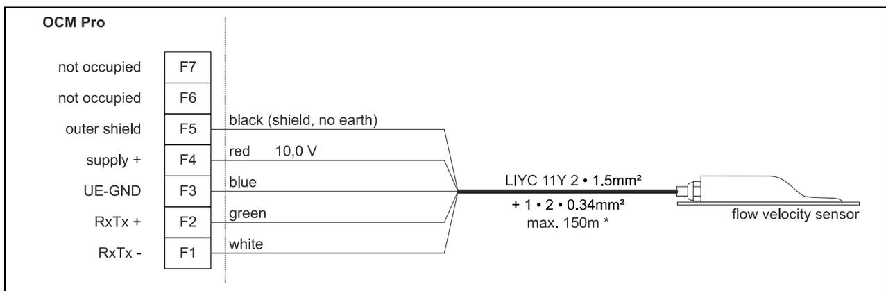
**Fig. 7-4** Connecting a second velocity sensor to the OCM Pro type M4W0
