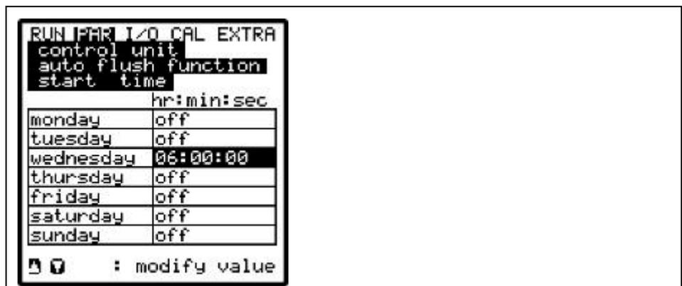
Fig. 9-92 Setting the flush start time
