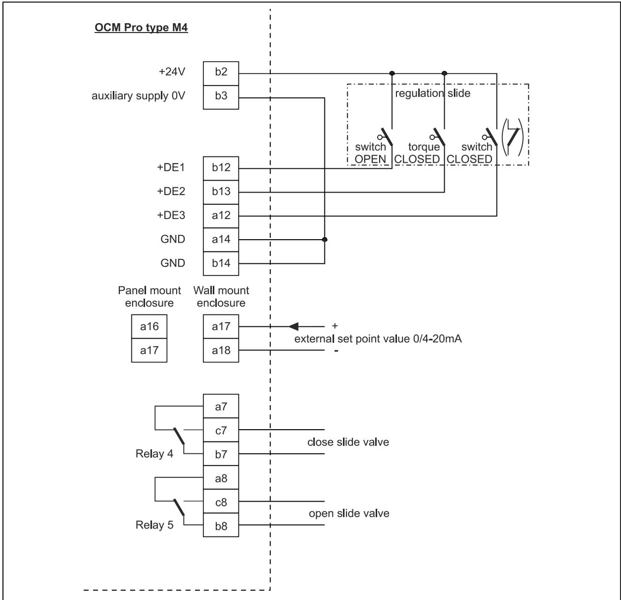
Fig. 7-39 Regulator mode wiring diagram
