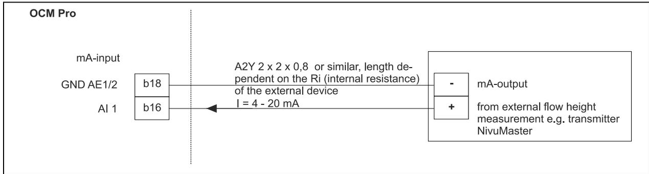
**Fig. 7-14 Connecting external level measurement from NivuMaster to type W0**
