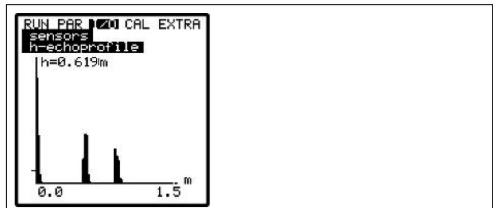
Fig. 9-135 Display echo profile with sensor type POA/OCL
