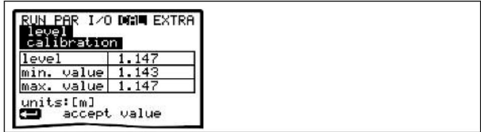
Fig. 9-149 Adjusting the level measurement
