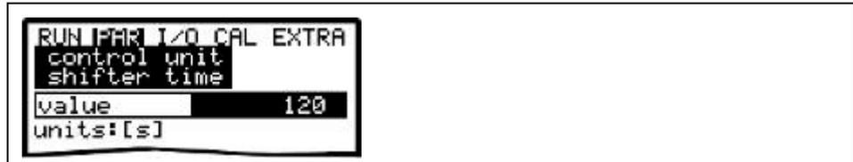
Fig. 9-86 Setting the shifter time
