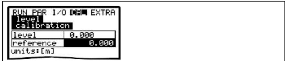
Fig. 9-150 Entering the correct filling level
