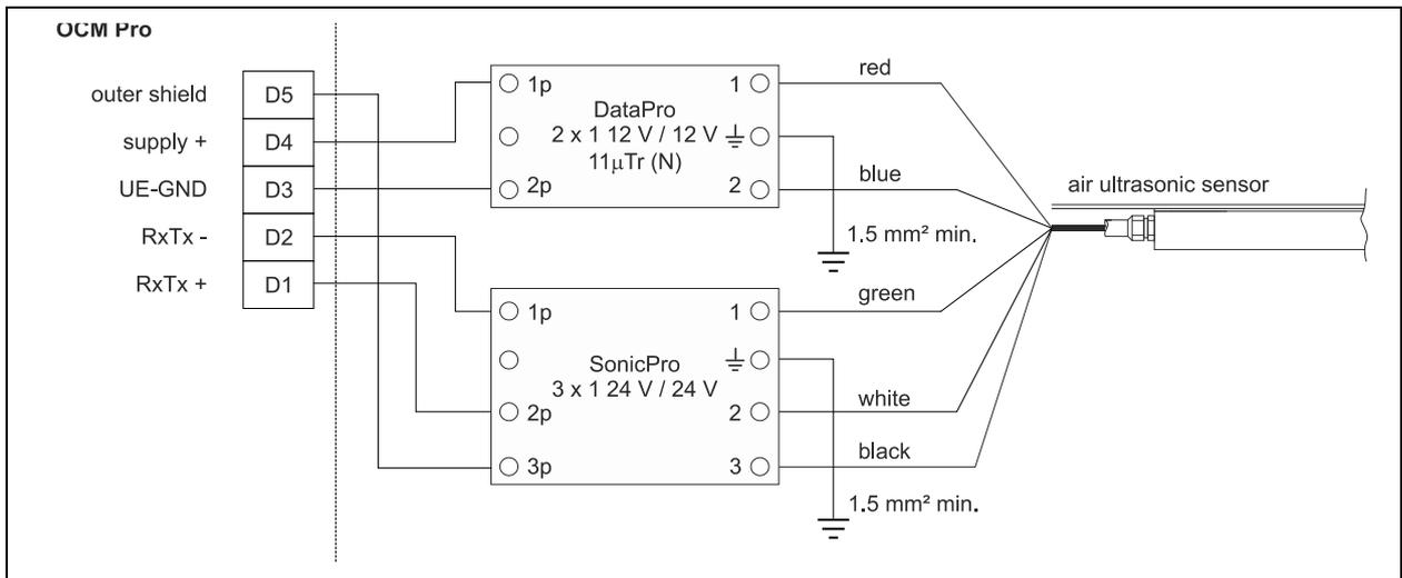
**Fig. 7-17** Overvoltage protection air-ultrasonic sensor, type OCL, wall mount enclosure
