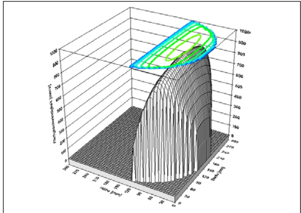
**Fig. 6-12 Computed 3-dimensional flow profile**
