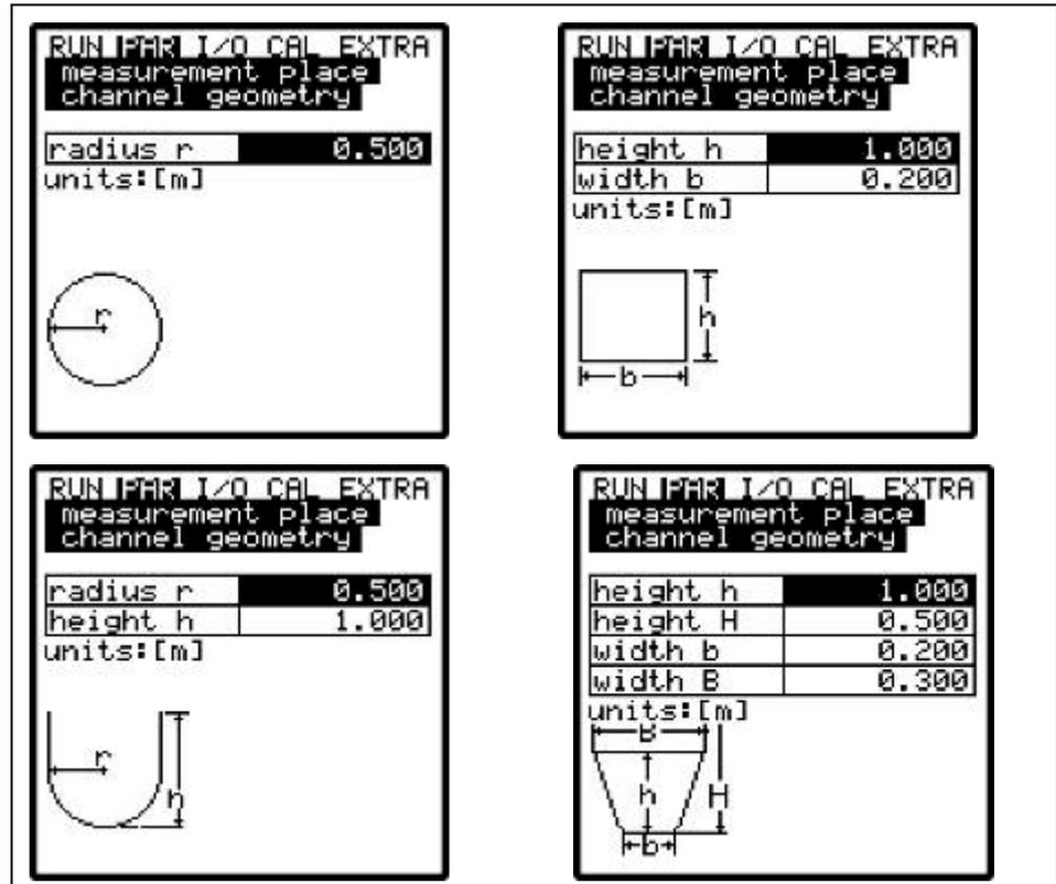
Fig. 9-26 Screens showing various channel dimensions
