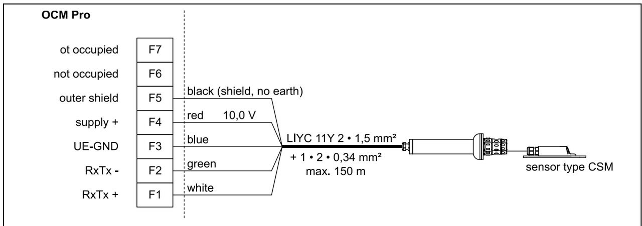
**Fig. 7-7 Connection 2, electronic box Type EBM with water-ultrasonic sensor Type CSM to Type M4W0**
