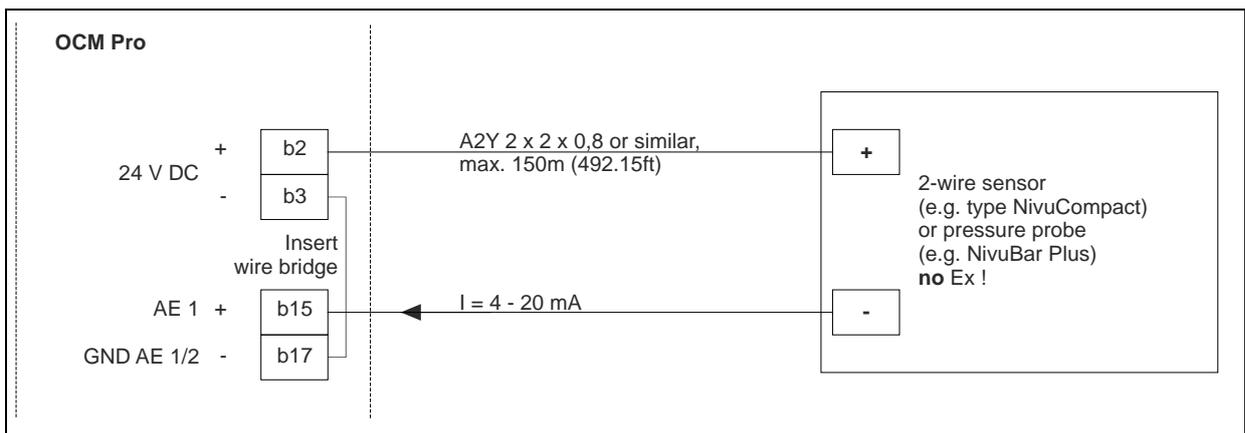
**Fig. 7-30 Connecting a 2-wire sensor for level measurement to type F0**
