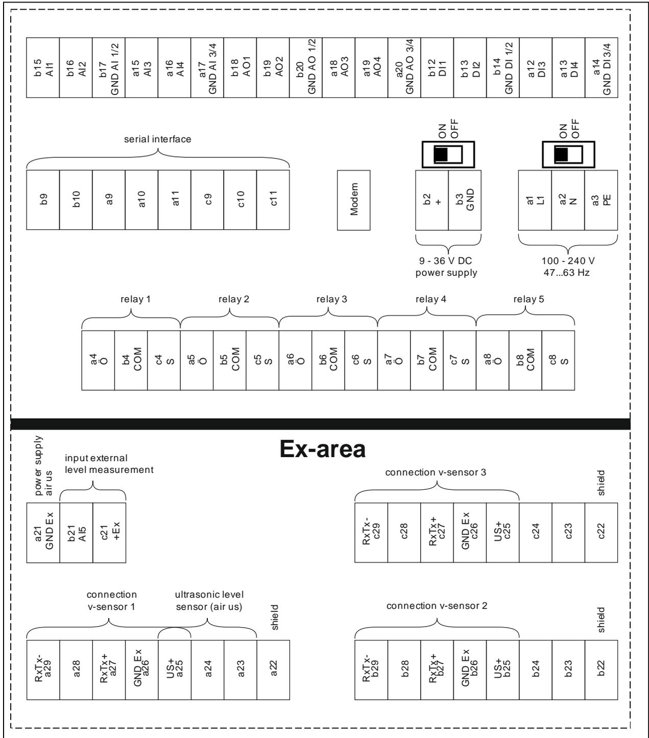
Fig. 7-19 Wiring diagram OCM Pro CF panel mount enclosure
