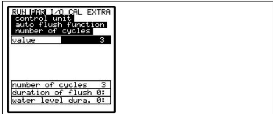
Fig. 9-93 Setting the number of cycles (flush events)
