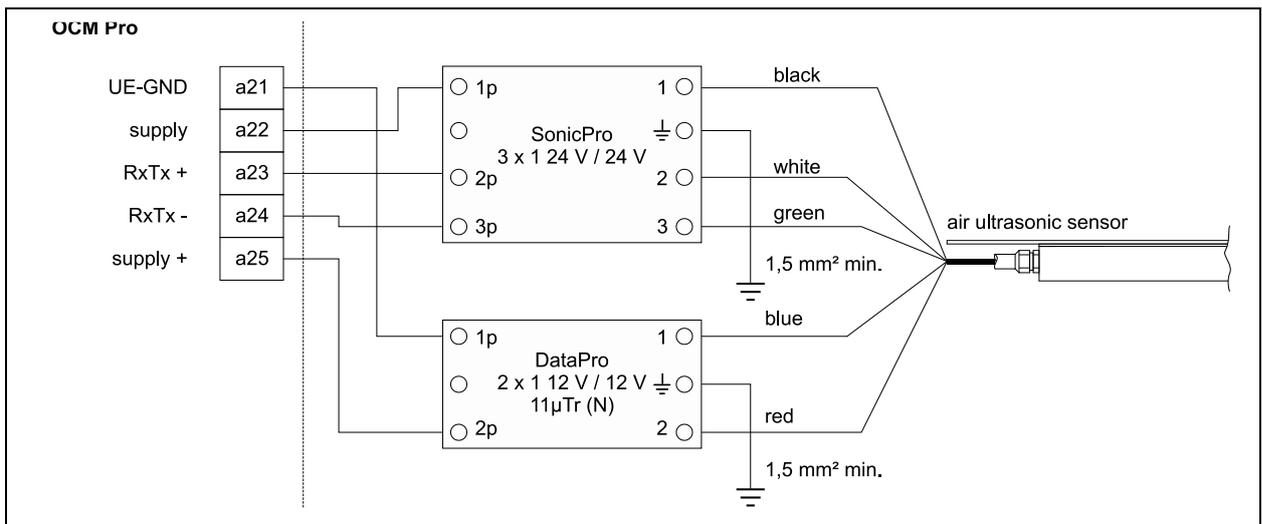
**Fig. 7-34** Overvoltage protection air-ultrasonic sensor type OCL, panel mount enclosure
