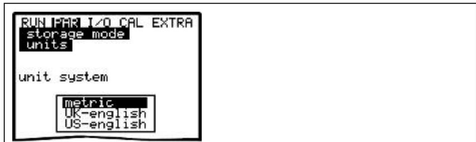
Fig. 9-106 Selecting the unit system in storage mode
