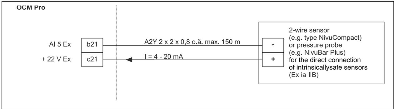
**Fig. 7-29 Connecting a 2-wire sensor EX for level measurement to type F0**
