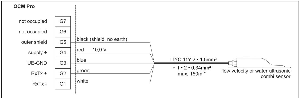
**Fig. 7-3** Connecting a flow velocity or water-ultrasonic combi sensor on the OCM Pro type S4W0 / M4W0
