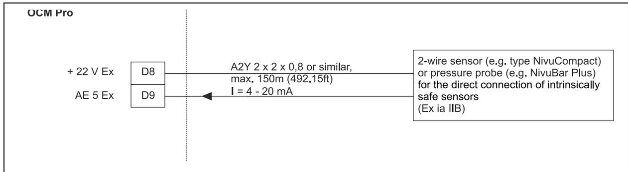
**Fig. 7-12 Connecting a 2-wire sensor (EX for level measurement)**
