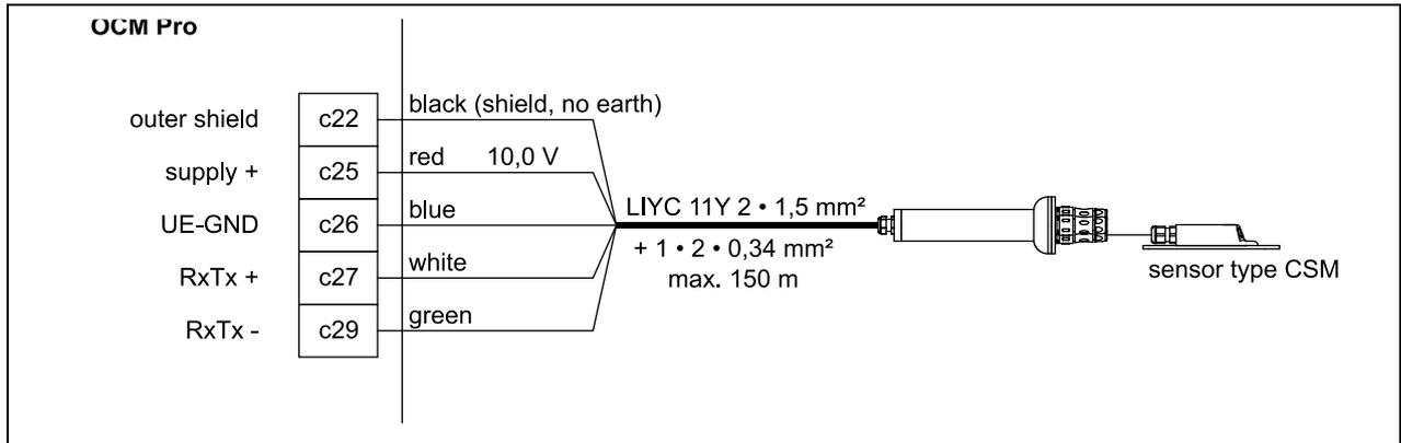
**Fig. 7-26 Connection 3, electronic box Type EBM with water-ultrasonic sensor Type CSM to Type M4F0**
