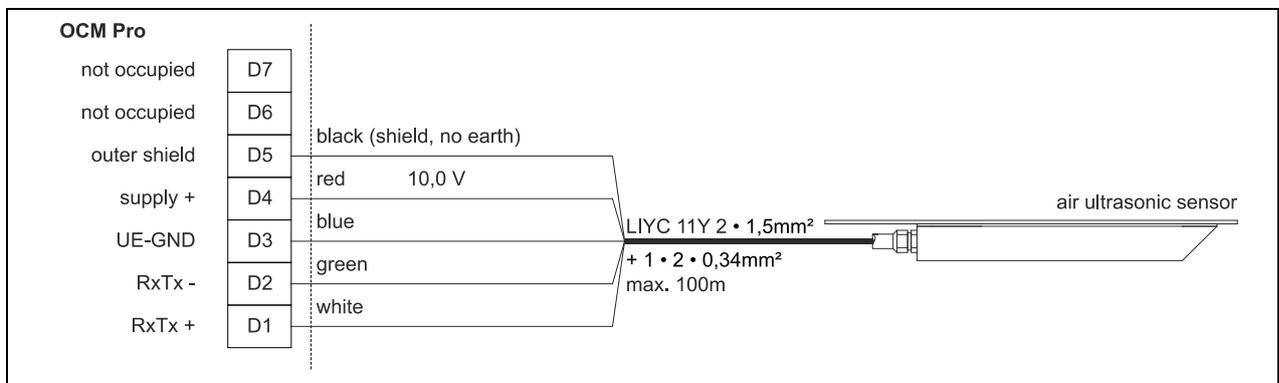
**Fig. 7-11 Connecting the air-ultrasonic sensor type LUS to type M4W0 / S4W0**
