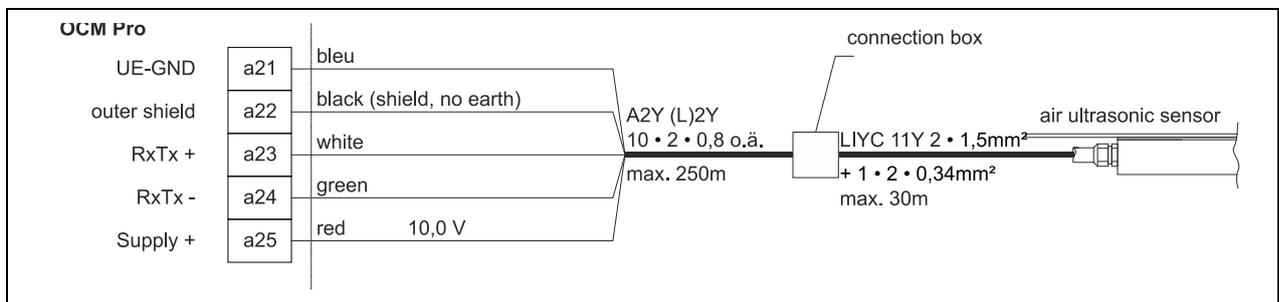
**Fig. 7-28 Connecting an air-ultrasonic sensor type OCL to type F0**
