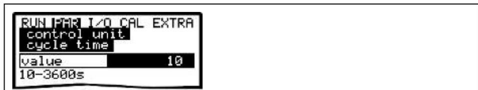
**Fig. 9-83 Setting the cycle time**
