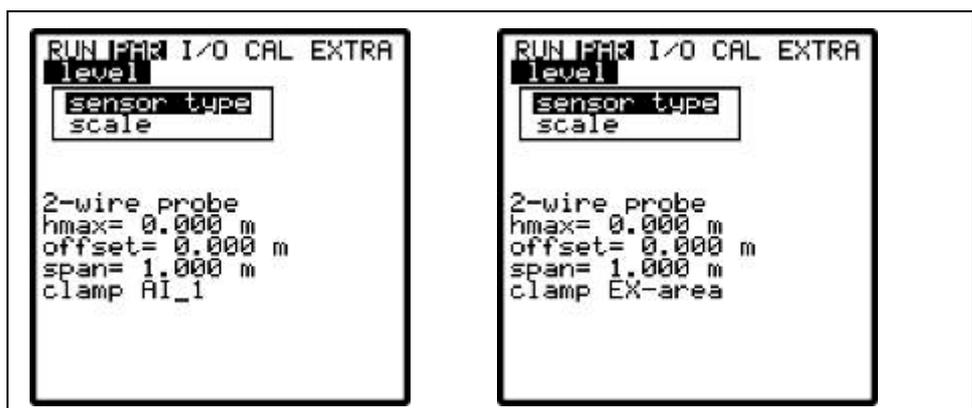
Fig. 9-50 Screen at 2-wire sensor Ex/non-Ex
