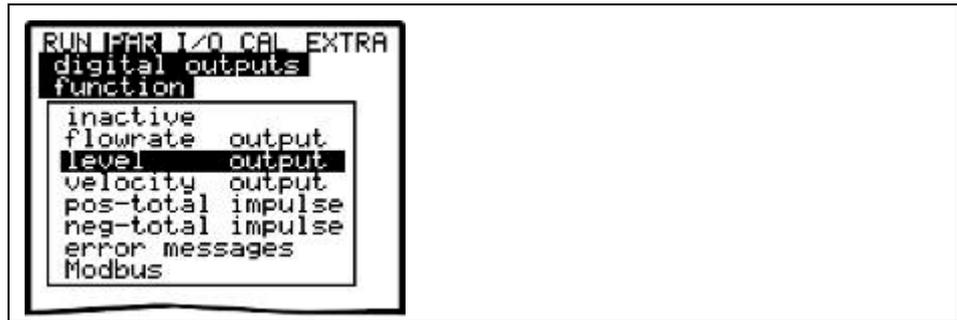
Fig. 9-73 Defining the relay function
