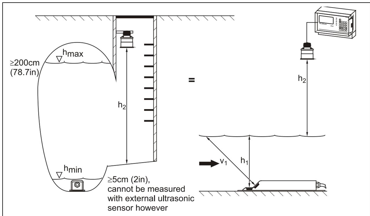
**Fig. 9-51 Application example for water-US + 2 Wire probe**
