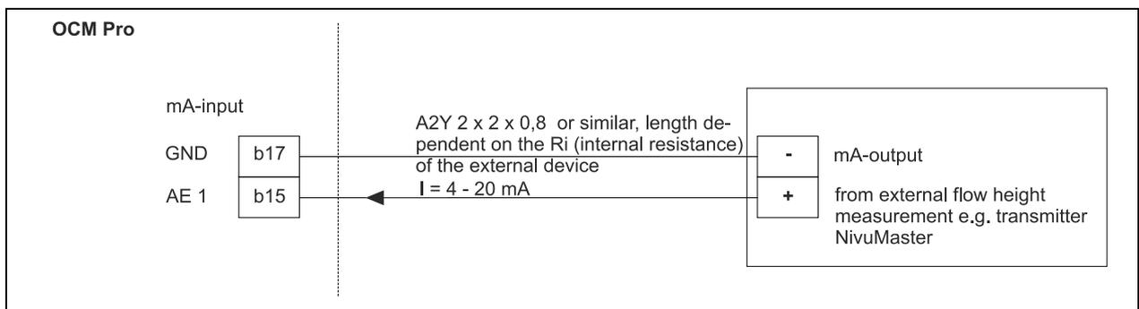
**Fig. 7-31 Connecting external level measurement to type F0**
