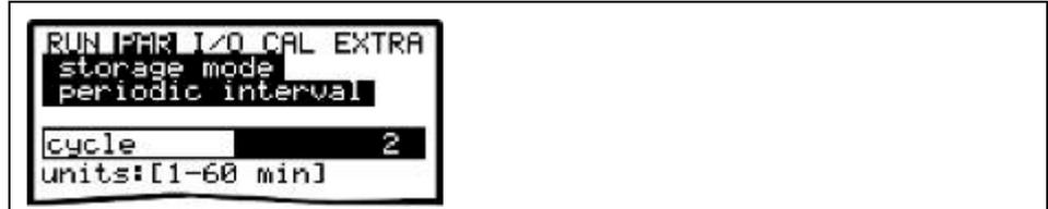
**Fig. 9-104 Entering the storage cycle**
