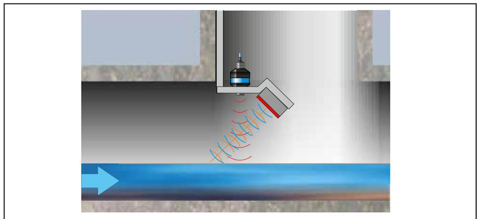
**Fig. 6-13 Measurement using the surface radar**
