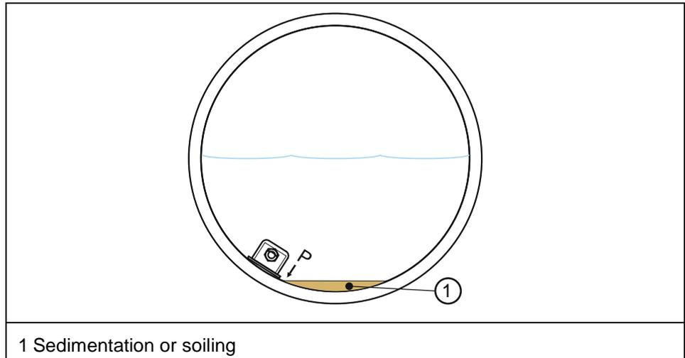
**Fig. 9-37 Sensor type 5: internal pressure**
