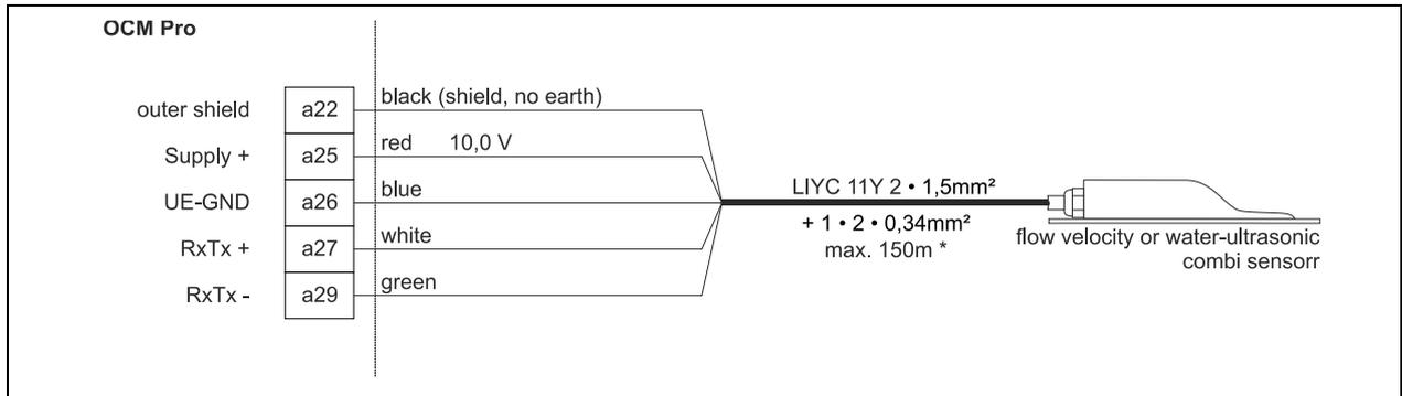
**Fig. 7-20 Connecting a flow velocity or water-ultrasonic combi sensor to the OCM Pro CF, type S4F0 / M4F0**
