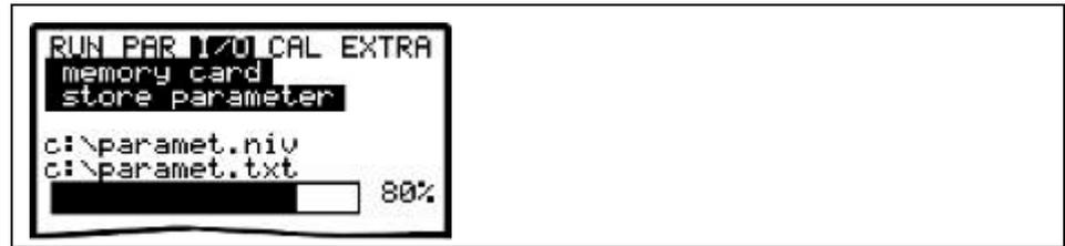
**Fig. 9-144 Saving parameters on memory card**
