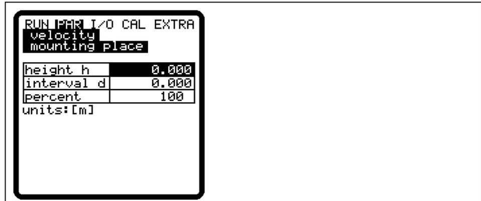
Fig. 9-63 Individual value assignment of flow velocity sensors
