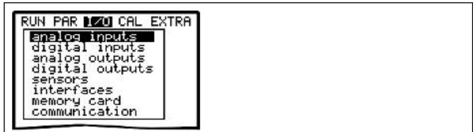
Fig. 9-123 I/O-submenu
