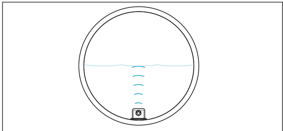
**Fig. 9-34 Sensor type 2: water-ultrasonic**
