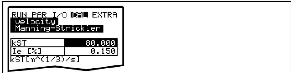
Fig. 9-155 Manning Strickler v-crit determination
