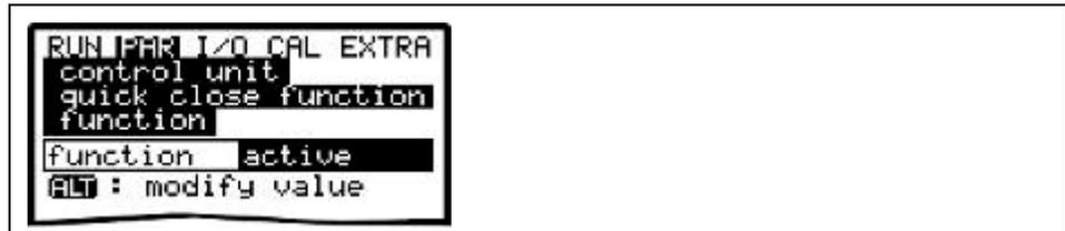
Fig. 9-87 Enabling quick close function
