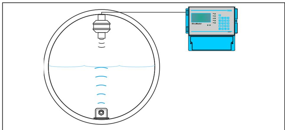
**Fig. 9-38 Sensor type 3: 2-wire probe**
