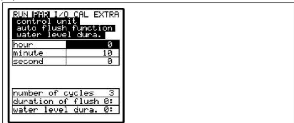
Fig. 9-95 Setting water level duration
