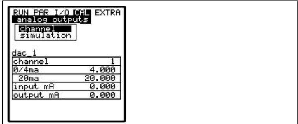
Fig. 9-156 Selecting the analog output simulation
