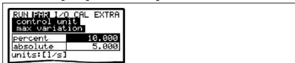
**Fig. 9-84 Setting permissible control deviations**
