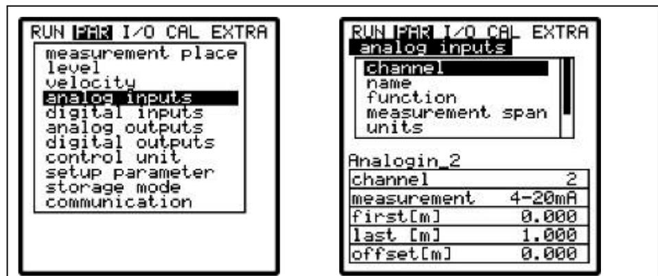
Fig. 9-64 Analog inputs – submenu
