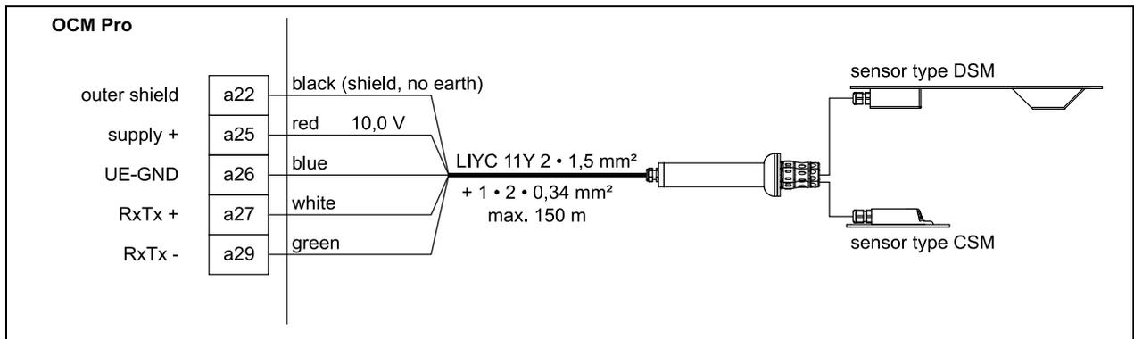
**Fig. 7-24 Connection electronic box Type EBM with water-ultrasonic sensor Type CSM and air-ultrasonic sensor Type DSM to Type S4F0 / M4F0**
