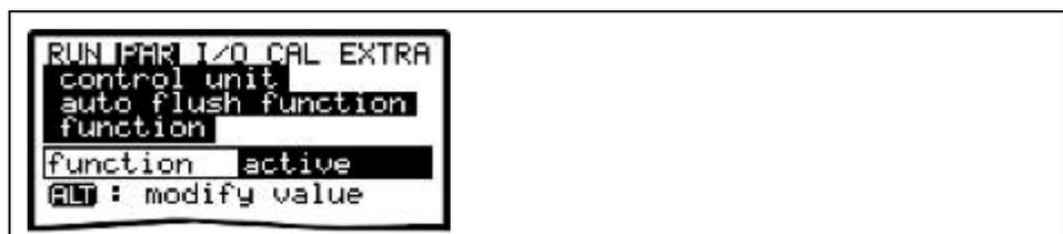
Fig. 9-89 Enabling the flush function
