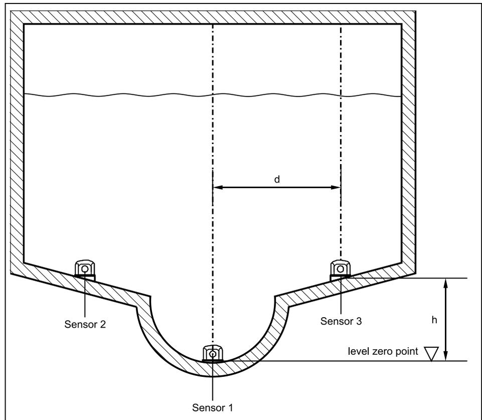
**Fig. 9-62 Sensor Assignment if using multiple v-sensors**
