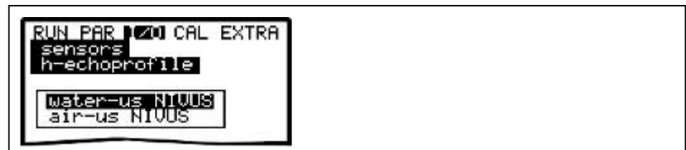
Fig. 9-134 Selecting level measurement echo profile
