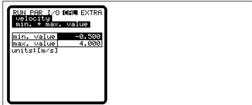
Fig. 9-152 Flow velocity measurement range
