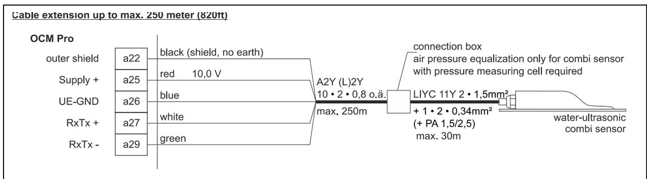
**Fig. 7-27 Connecting a flow velocity sensor with integrated pressure measurement cell to type F0**
