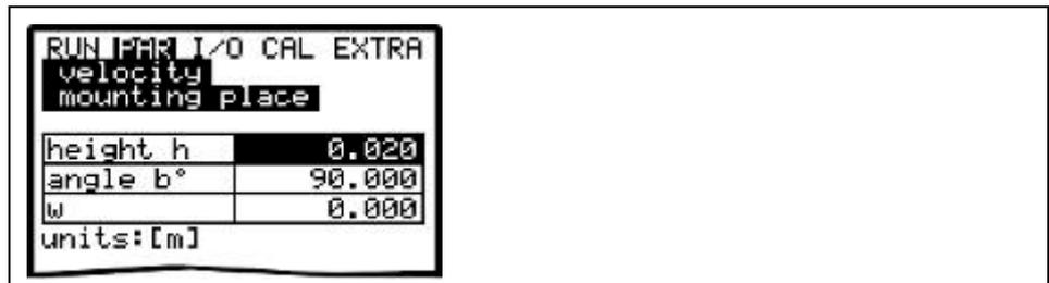
>height h< is the distance from the channel bottom to the bottom edge of the sensor ground plate.
