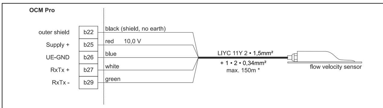
**Fig. 7-22 Connecting a second flow velocity sensor to type M4F0**
