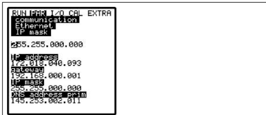
Fig. 9-114 Setting the IP address manually
