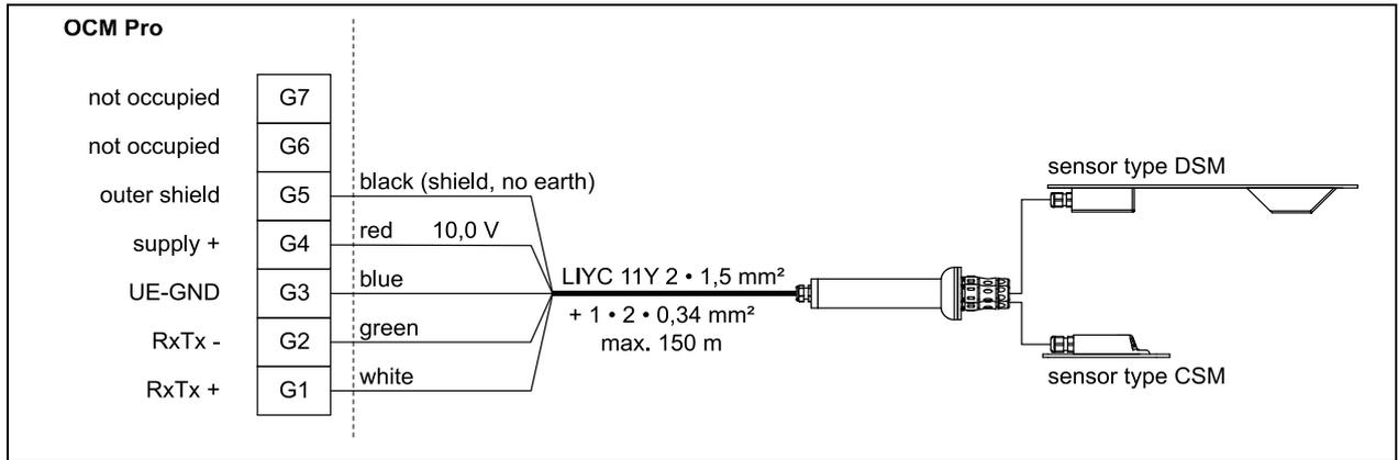
**Fig. 7-6 Connection electronic box Type EBM with water-ultrasonic sensor Type CSM and air-ultrasonic sensor Type DSM to Type S4W0 / M4W0**
