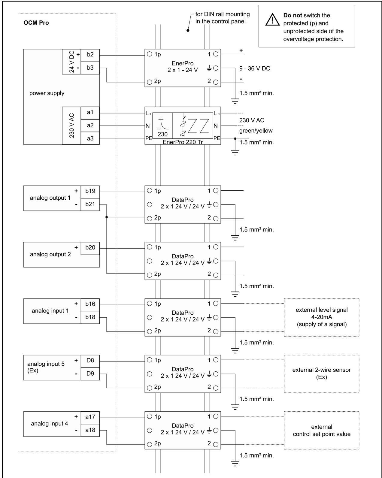
**Fig. 7-15 Wall mount enclosure - connecting the overvoltage protection for power supply and analog inputs and outputs**
