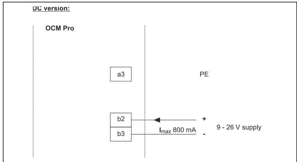
Fig. 7-37 DC model power supply
