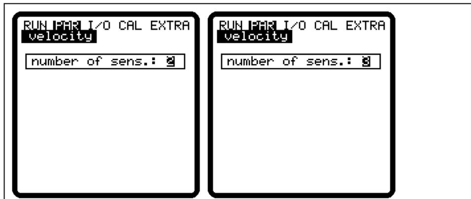
Fig. 9-59 Selecting the number of flow velocity sensors
