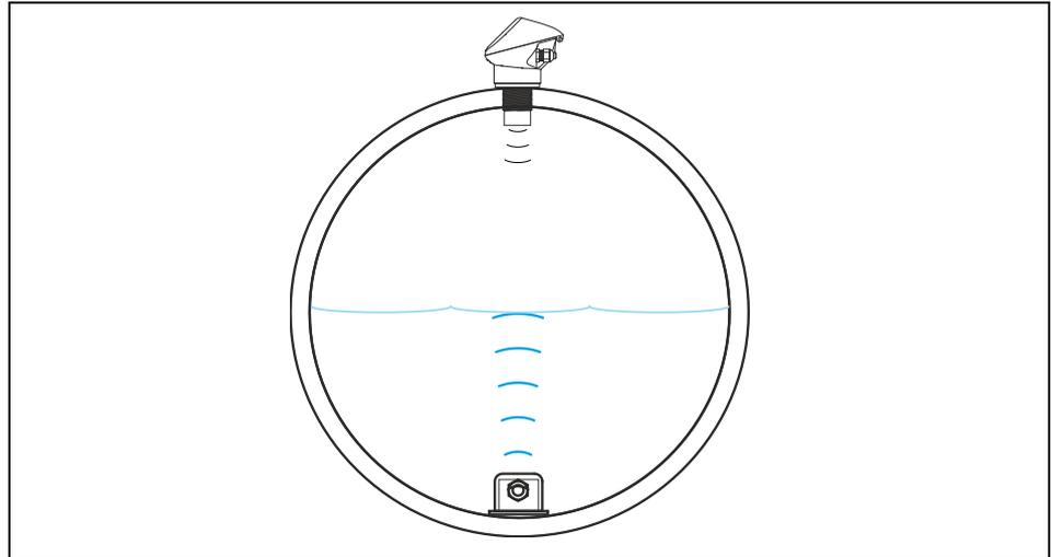
**Fig. 9-42 Water-ultrasound + 2-wire probe**
