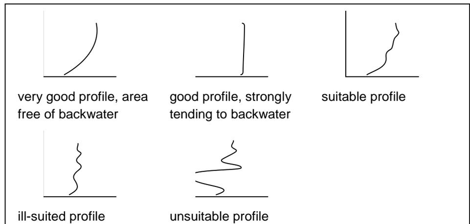
**Fig. 9-7 Flow velocity profiles**
