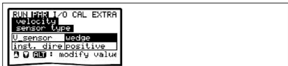
Fig. 9-61 Select sensor type and mounting position
