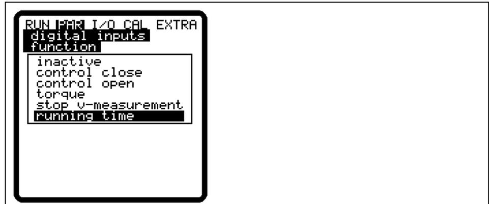
**Fig. 9-68 Digital input functions**
