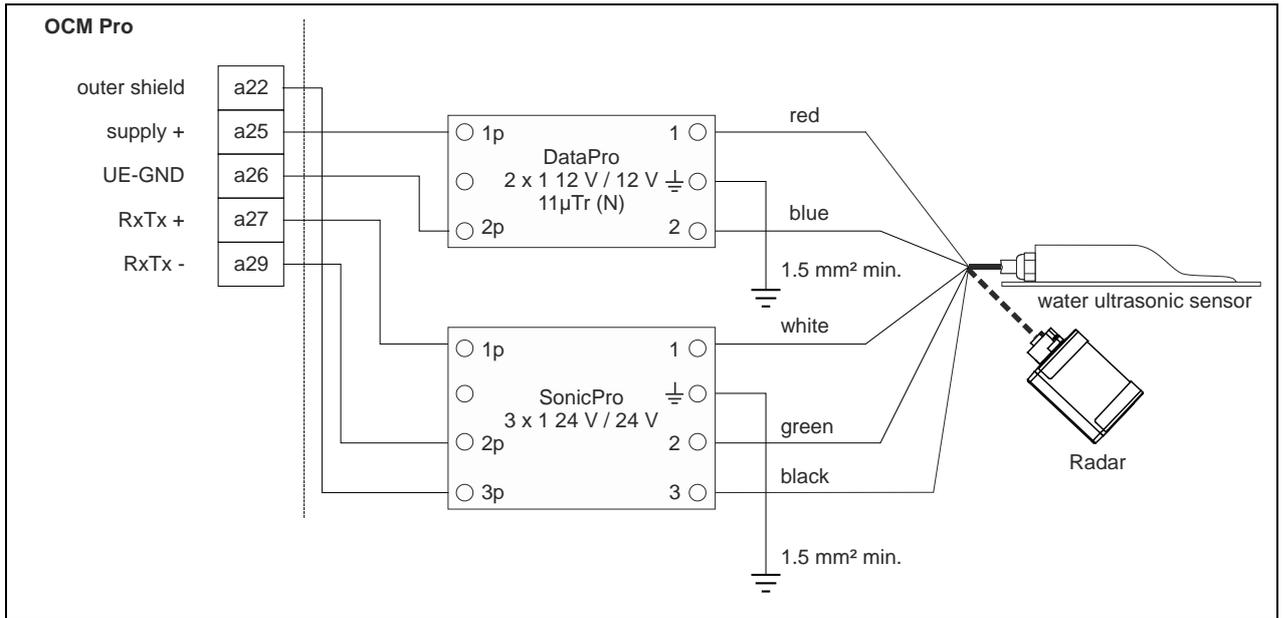
**Fig. 7-33** Overvoltage protection water-ultrasonic sensor or electronic box or OFR radar, panel mount enclosure
