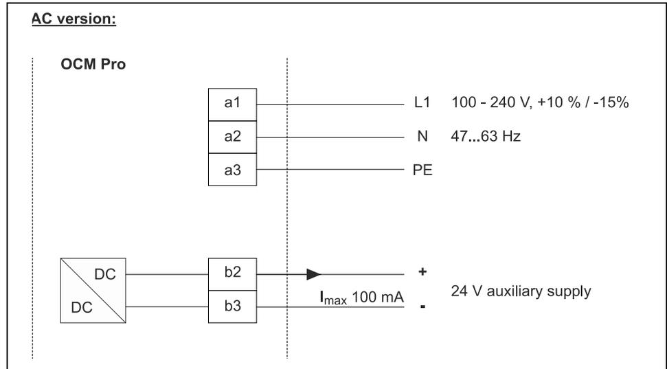
Fig. 7-36 AC model power supply
