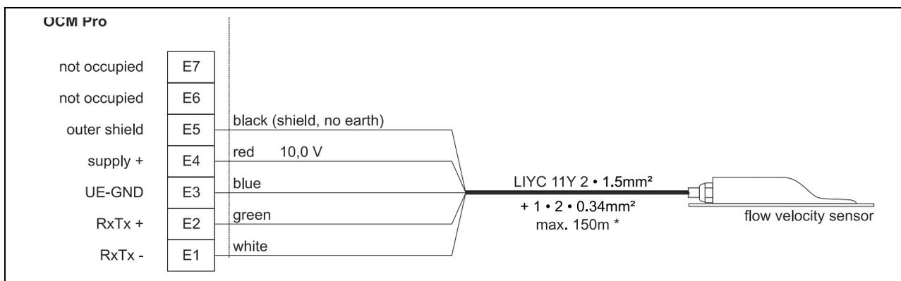
**Fig. 7-5** Connecting a third velocity sensor to the OCM Pro type M4W0
