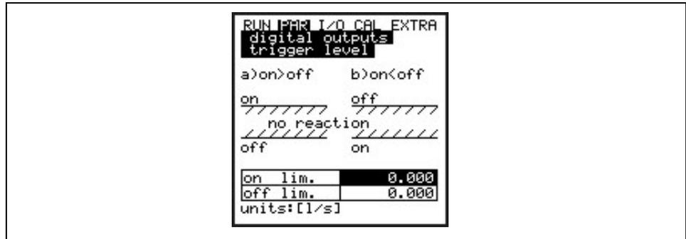
**Fig. 7-3 Relay trigger level settings**
