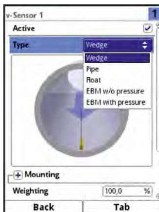
Fig. 23-15 Selection menu flow velocity sensors
