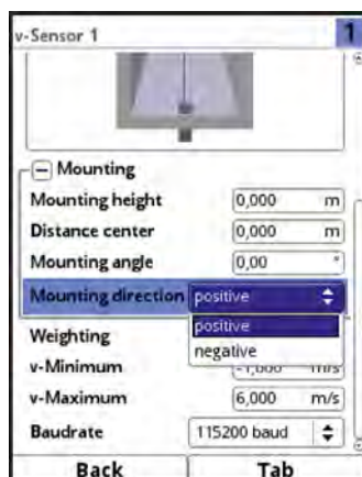
Fig. 23-21 Sensor installation direction altering options
