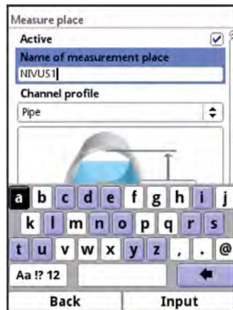
Fig. 23-1 Entering the name of the measurement place
