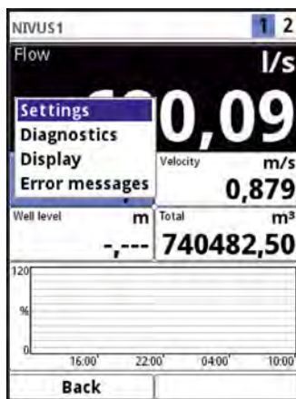
Fig. 20-2 Flow volume section selected
