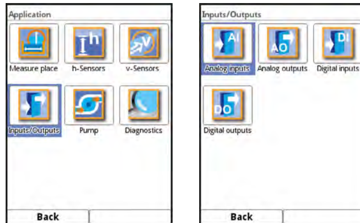
Fig. 23-25 Selection of inputs and outputs
