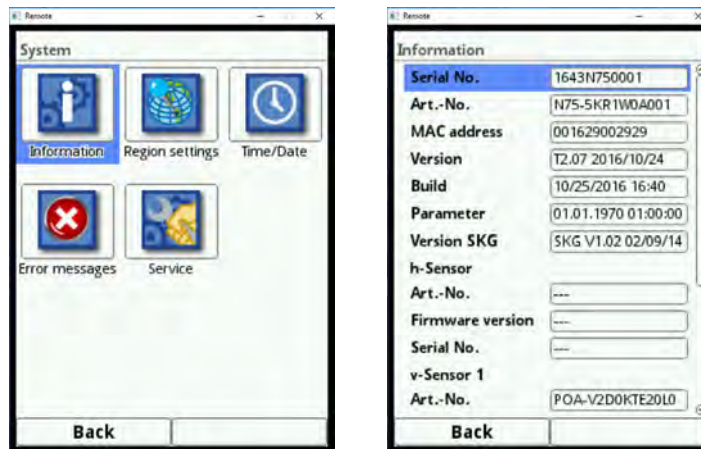
Fig. 25-1 System submenu/system information
