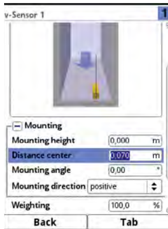
Fig. 23-20 Entering sensor positions related to application centre
