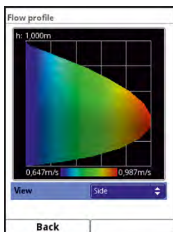
Fig. 13-4 Determined flow profile
